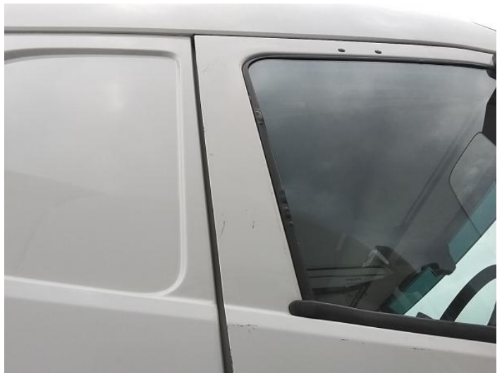
12: Door osf Scratched Over 25mm Thru Paint
