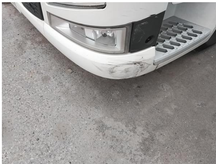
2: Bumper Front Scratched Over 100mm Thru Paint
