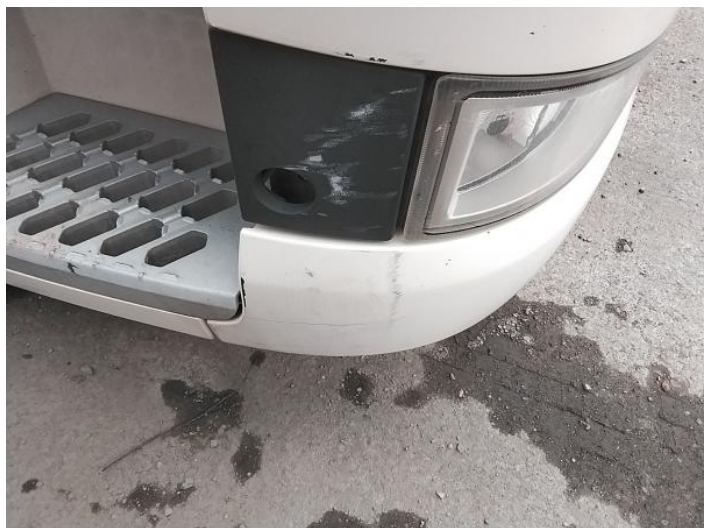
14: Bumper Front Scratched Over 100mm Thru Paint
