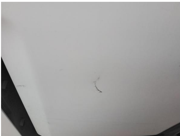
4: Door nsf Dented With Paint Damage
