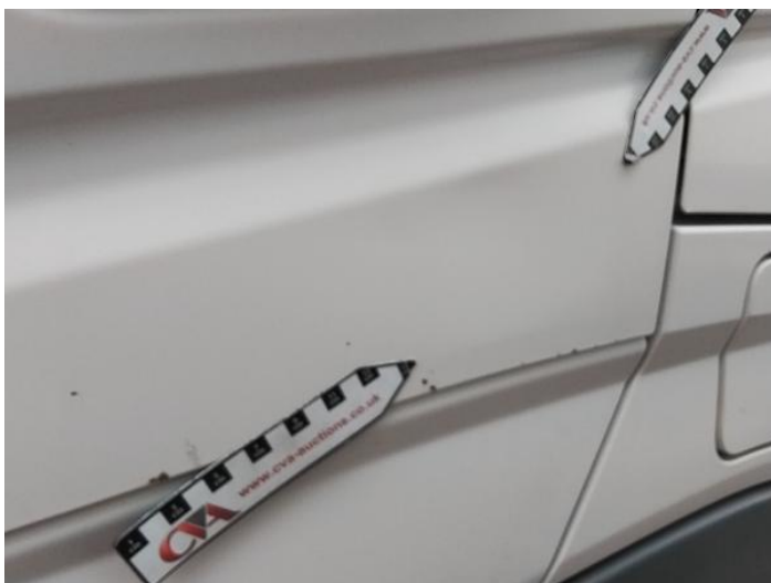
6: Door nsf Dented Over 30mm
