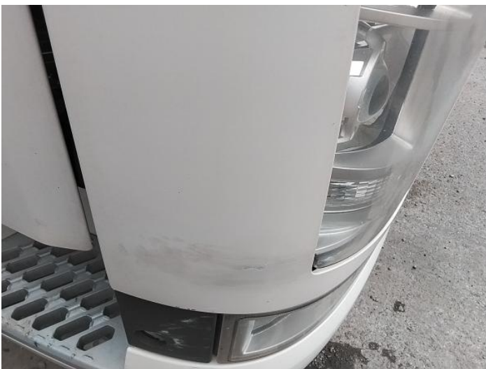
13: Panel Front Poor Previous Repair Poor Colour
