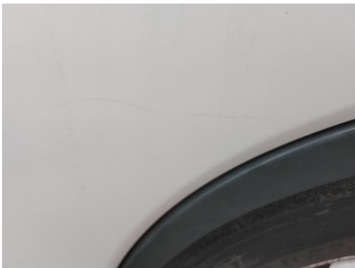
7: Door nsf Scratched Over 25mm Not Thru Paint
