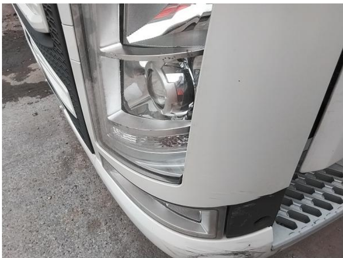
3: Panel Front Scratched Over 25mm Thru Paint
