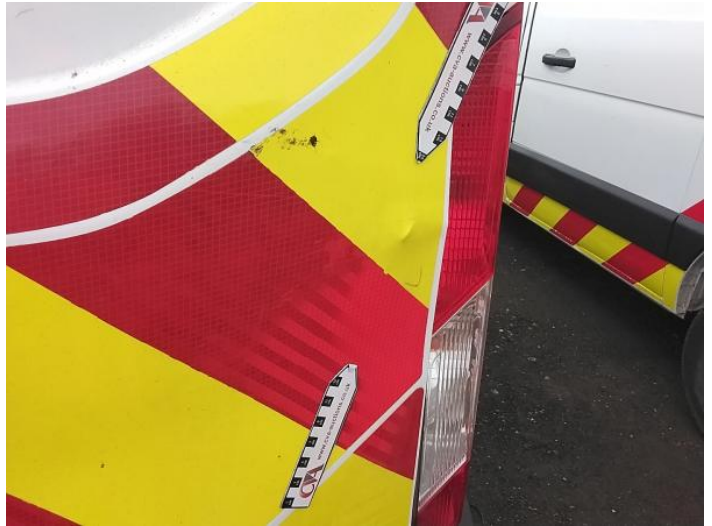
40: Door osr Dented Over 30mm
