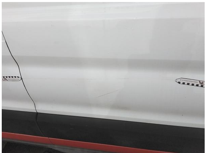
50: Qtr Panel osr Scratched Over 25mm Thru Paint
