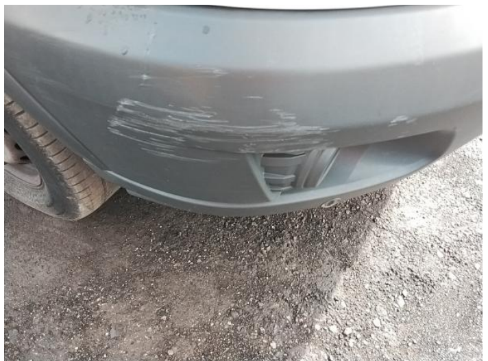
56: Bumper Front Scratched Over 100mm Thru Paint
