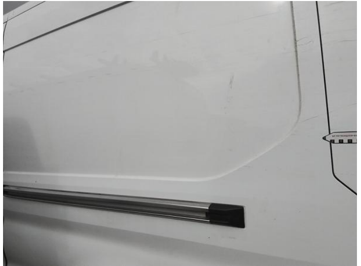
28: Qtr Panel nsr Scratched Over 25mm Thru Paint
