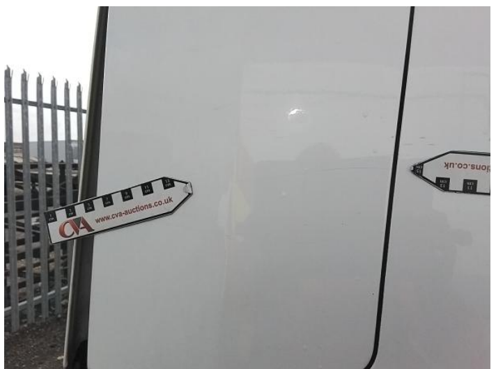
44: C Post os Scratched Over 25mm Thru Paint
