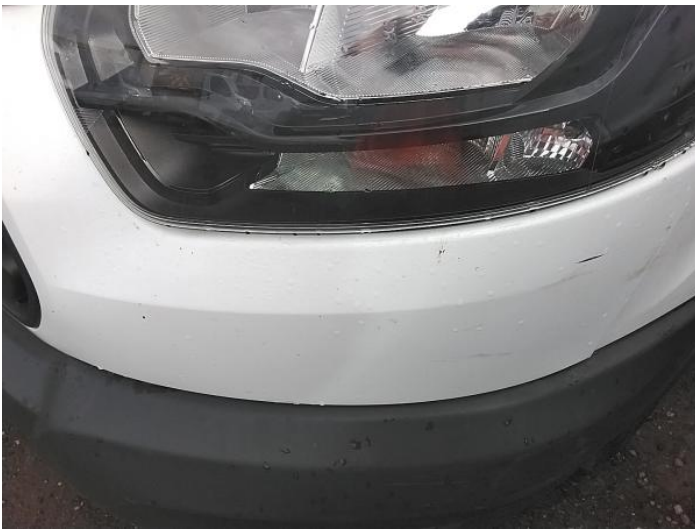
5: Panel Front Scratched Over 25mm Thru Paint
