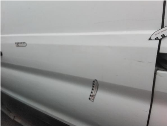
21: Qtr Panel nsr Dented Over 30mm
