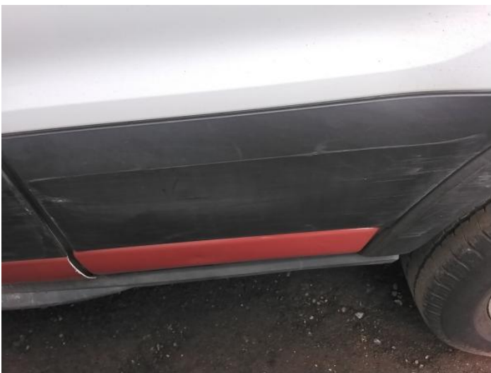
31: Qtr Panel Moulding ns Scuffed (Unpainted) Over 100mm
