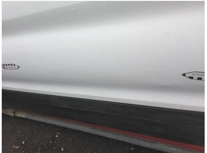
24: Qtr Panel nsr Scratched Over 25mm Thru Paint
