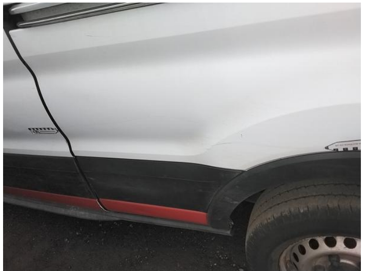
30: Qtr Panel nsr Scratched Over 25mm Thru Paint
