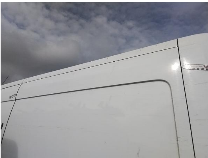
25: Qtr Panel nsr Scratched Over 25mm Thru Paint
