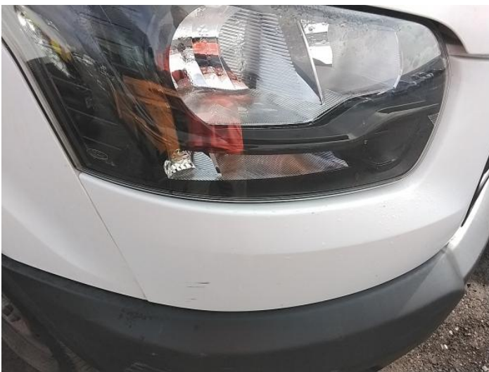
55: Panel Front Scratched Over 25mm Thru Paint
