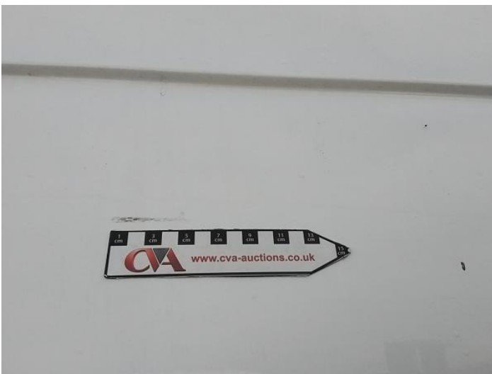
49: Qtr Panel osr Scratched Over 25mm Not Thru Paint
