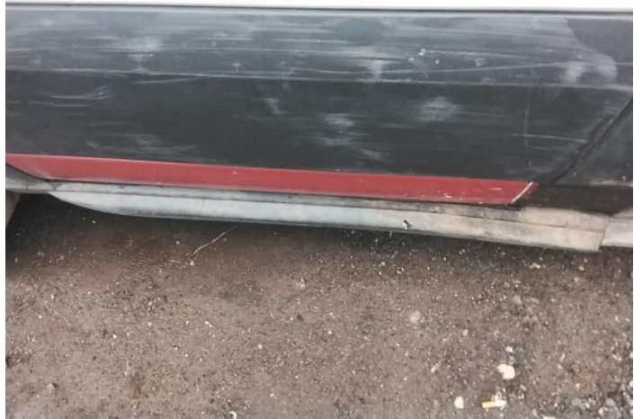
12: Door Moulding nsf Scuffed (Unpainted) Over 100mm
