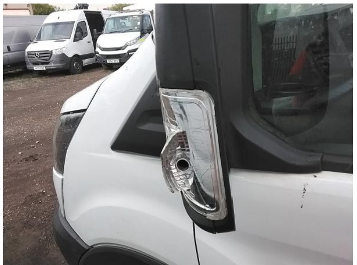
8: Door Mirror Assy nsf Broken Replace
