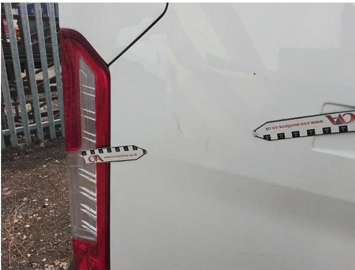
47: Qtr Panel osr Scratched Over 25mm Thru Paint
