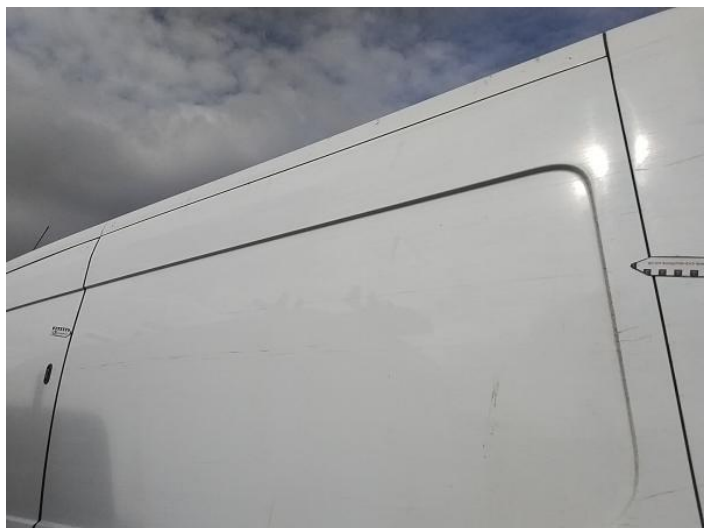
26: Qtr Panel nsr Scratched Over 25mm Thru Paint
