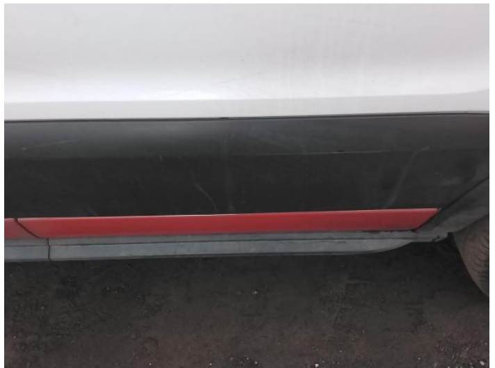
54: Door Moulding osf Scuffed (Unpainted) Over 100mm
