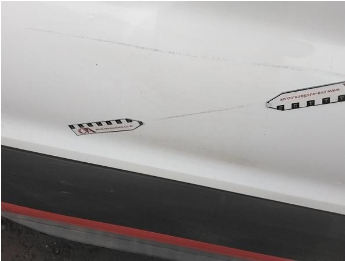
51: Qtr Panel osr Scratched Over 25mm Not Thru Paint
