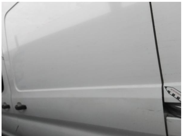
20: Qtr Panel nsr Scratched Over 25mm Thru Paint
