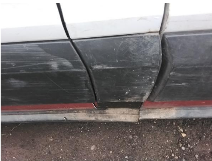
13: Door Moulding nsf Scuffed (Unpainted) Over 100mm
