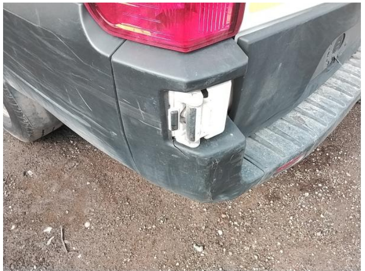
36: Bumper Rear Moulding Broken Replace
