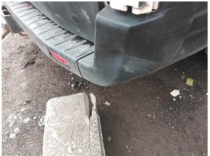
42: Bumper Rear Moulding Broken Replace
