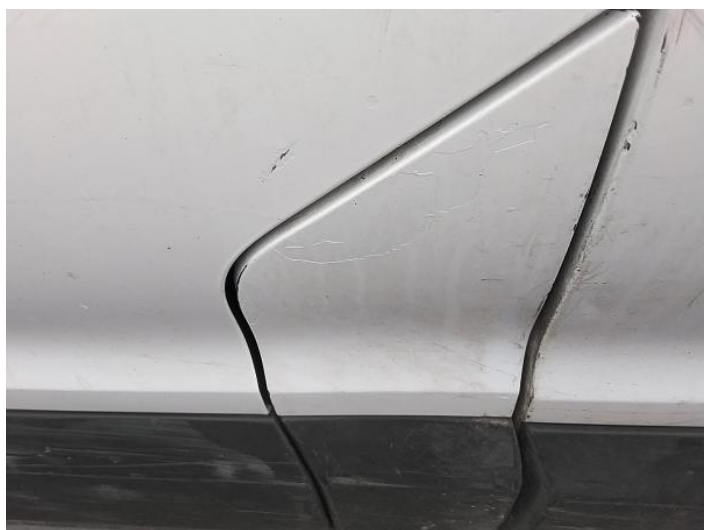
14: Fuel Flap Scratched Over 25mm Thru Paint
