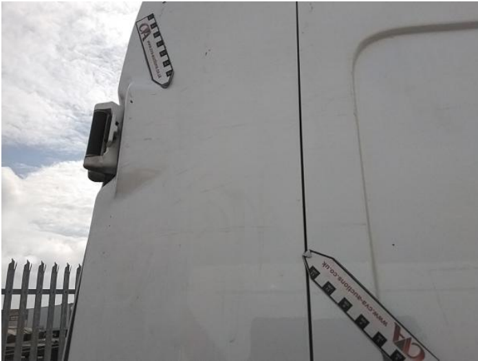
45: C Post os Scratched Over 25mm Thru Paint
