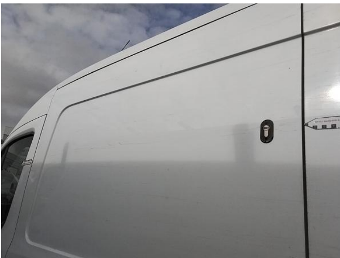
19: Qtr Panel nsr Scratched Over 25mm Thru Paint
