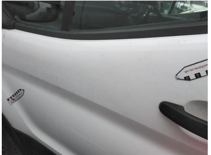
10: Door nsf Scratched Over 25mm Thru Paint
