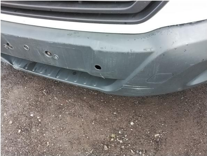
3: Bumper Front Scratched Over 100mm Thru Paint
