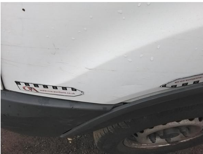
7: Wing nsf Dented Over 30mm
