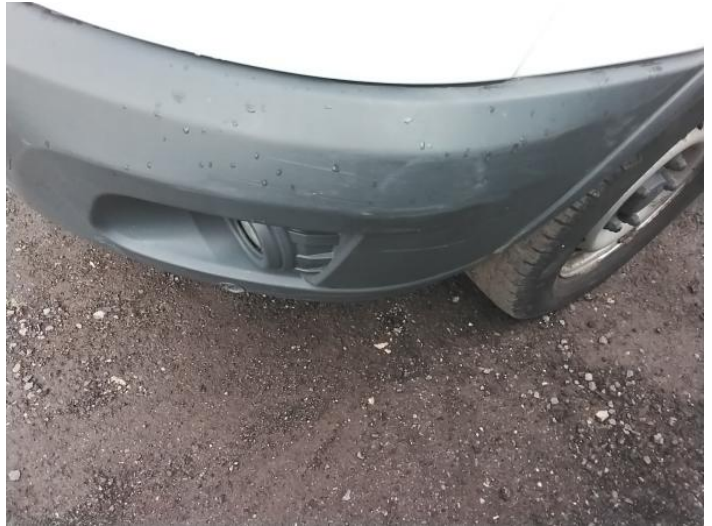
4: Bumper Front Scratched Over 100mm Thru Paint
