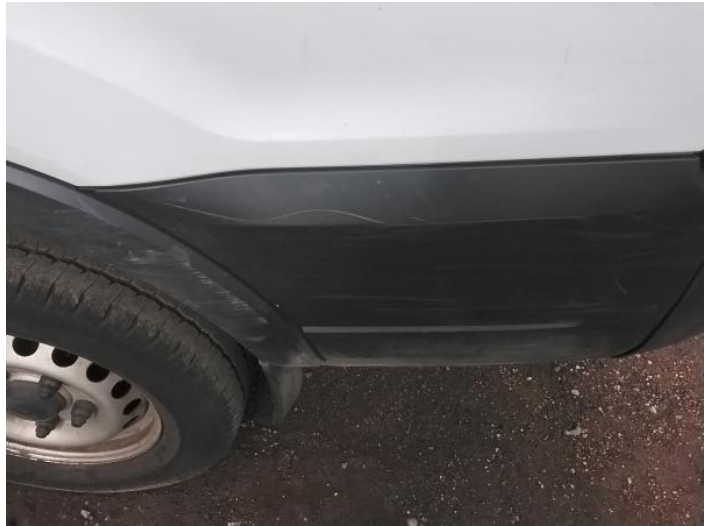
34: Qtr Panel Moulding ns Scuffed (Unpainted) Over 100mm
