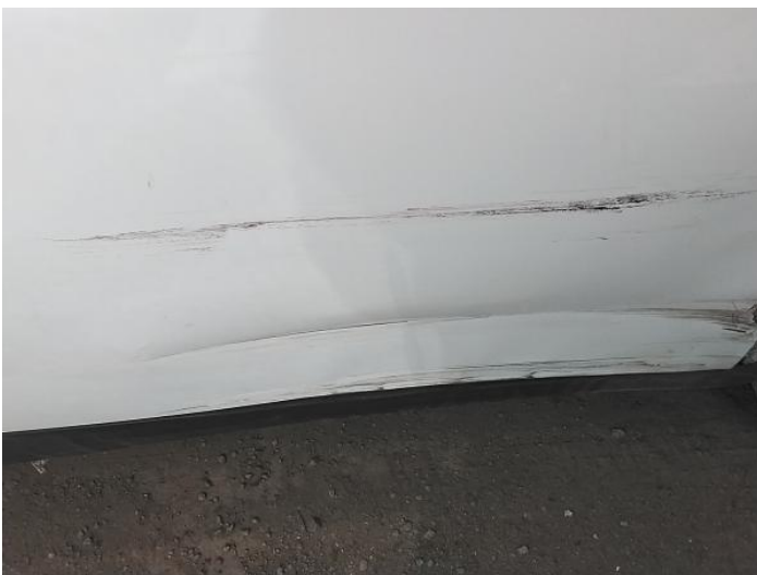
7: Qtr Panel nsr Dented With Paint Damage
