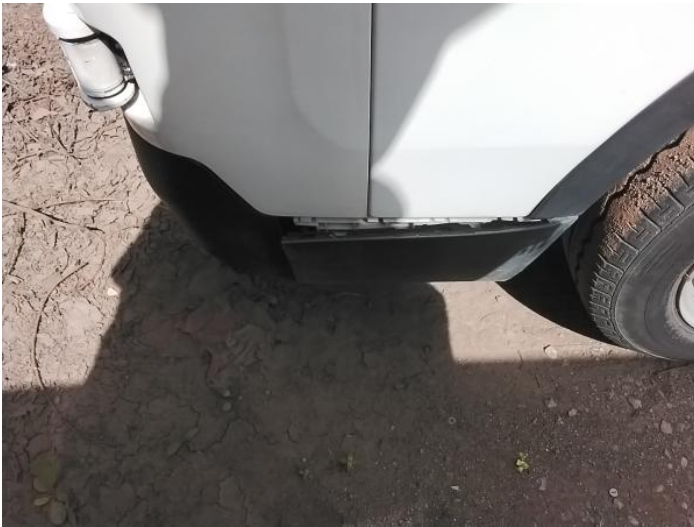
17: Qtr Panel Moulding os Broken Replace
