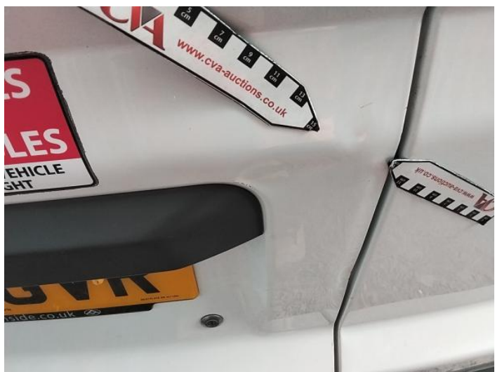
14: Door nsr Dented Over 30mm
