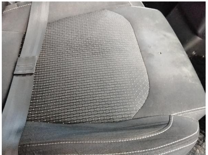
24: Seat Base Cover osf Burn Over 3mm
