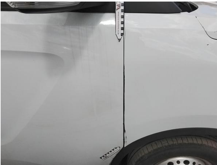
23: Door osf Dented Over 30mm
