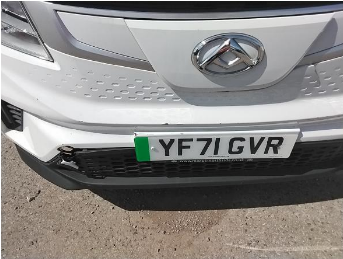
3: Panel Front Scratched Over 25mm Thru Paint
