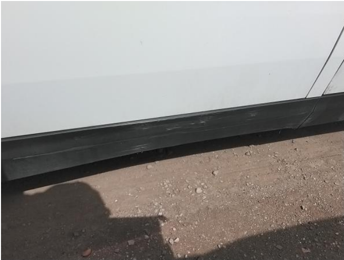
21: Qtr Panel Moulding os Scuffed (Unpainted) Over 100mm
