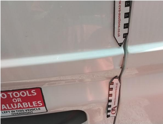
15: Door nsr Dented With Paint Damage
