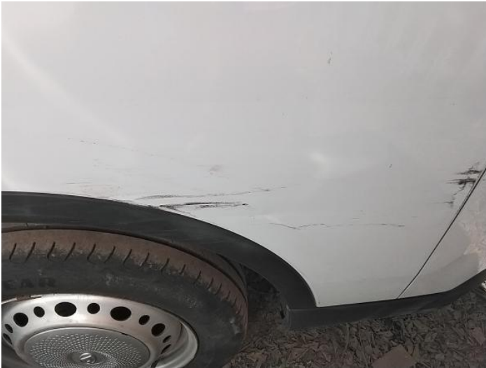
9: Qtr Panel nsr Dented With Paint Damage
