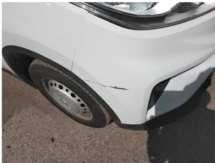
2: Panel Front Scratched Over 25mm Thru Paint
