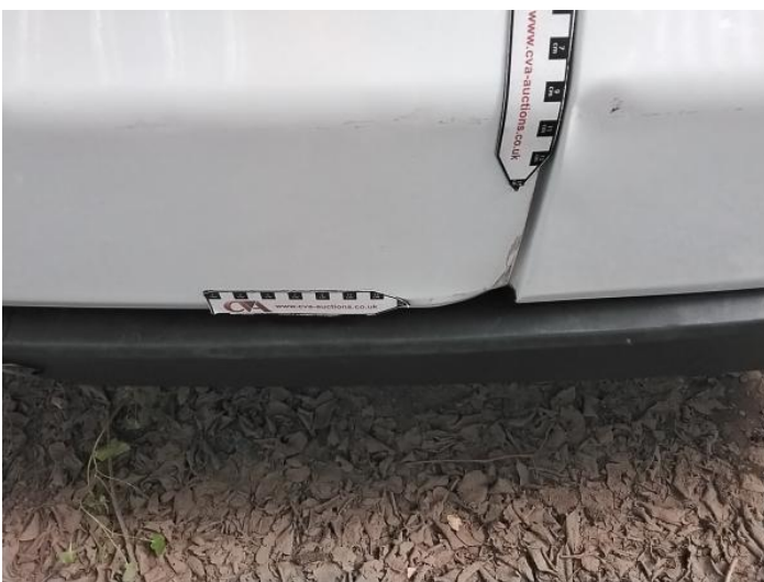
13: Door nsr Dented With Paint Damage
