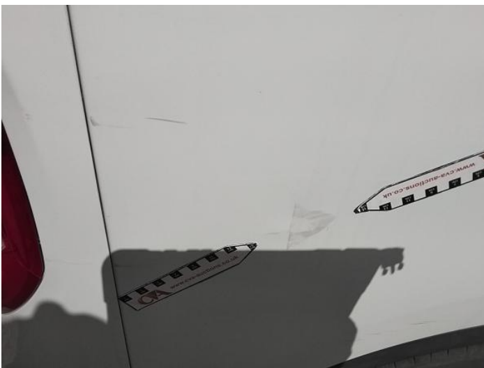
19: Qtr Panel osr Dented With Paint Damage
