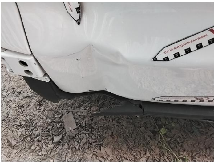
11: Door nsr Dented With Paint Damage
