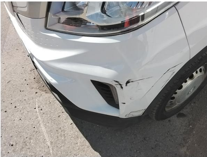
5: Panel Front Scratched Over 25mm Thru Paint
