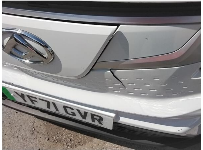
4: Panel Front Cracked Replace
