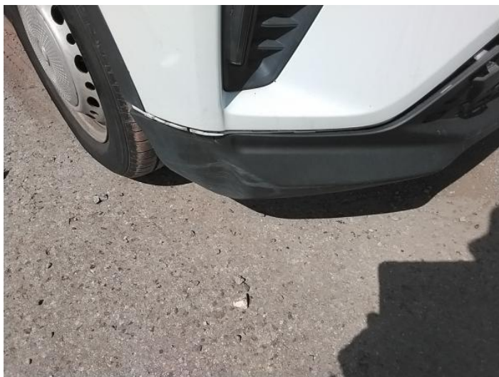
1: Bumper Front Cracked Over 25mm
