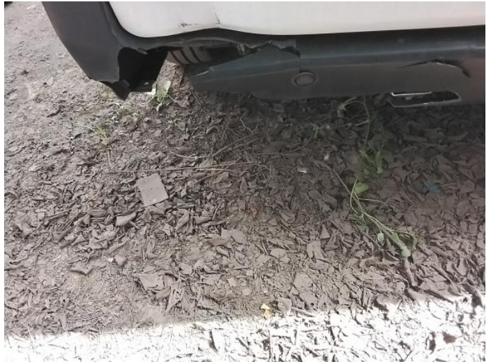
10: Bumper Rear Cracked Over 25mm
