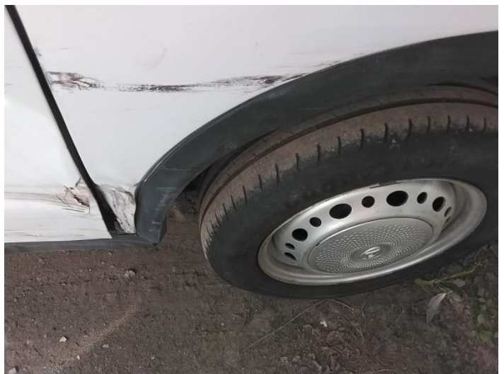
8: Qtr Panel nsr Dented With Paint Damage
