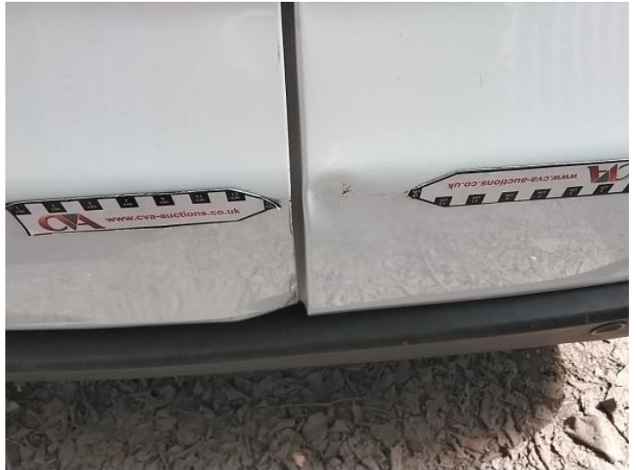
16: Door osr Dented With Paint Damage
