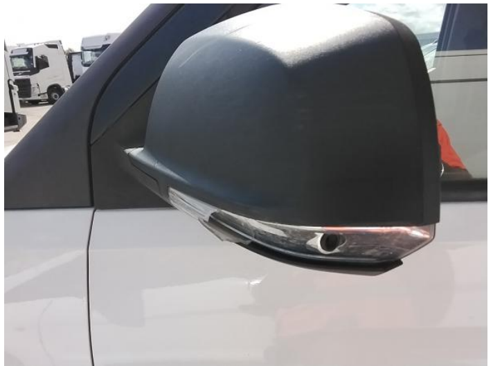
6: Door Mirror Assy nsf Broken Replace
