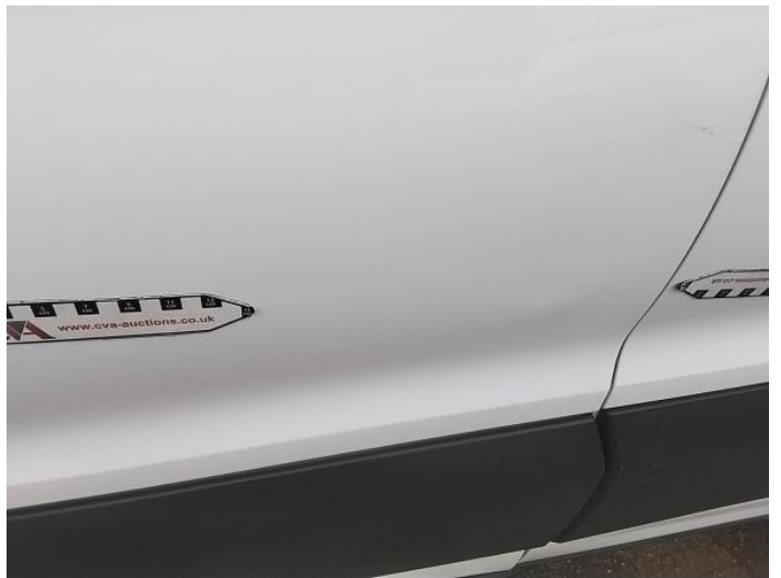
6: Qtr Panel nsr Dented Over 30mm
