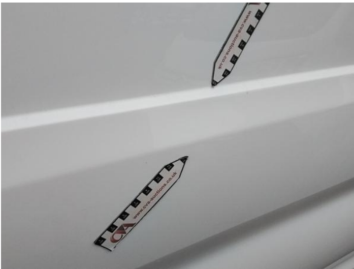
5: Qtr Panel nsr Dented Over 30mm
