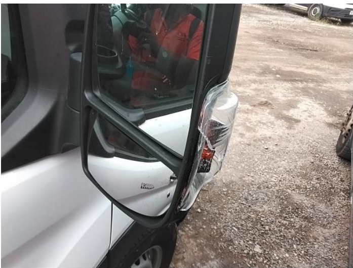
19: Door Mirror Assy osf Broken Replace
