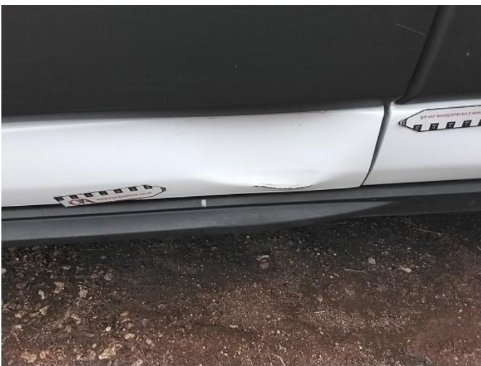
7: Qtr Panel nsr Dented With Paint Damage
