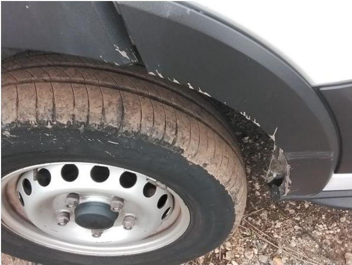
3: Door Moulding nsf Scuffed (Unpainted) UpTo 100mm
