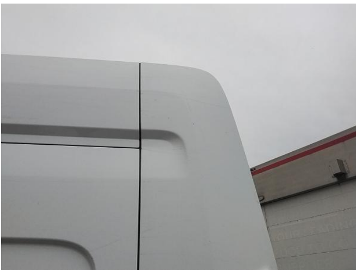
13: C Post ns Scratched Over 25mm Thru Paint
