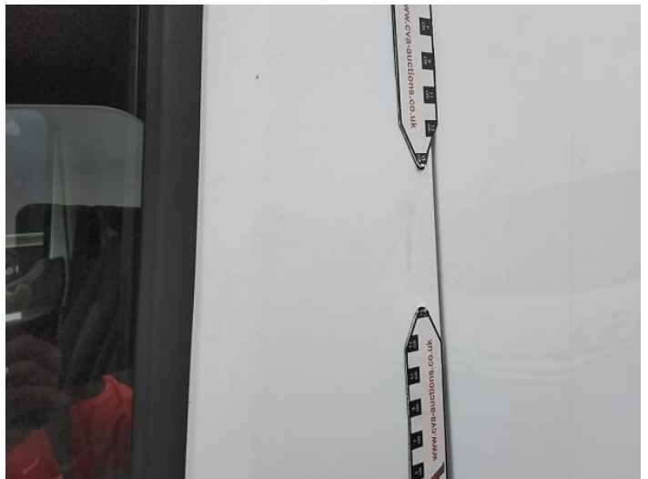
2: Door nsf Dented With Paint Damage
