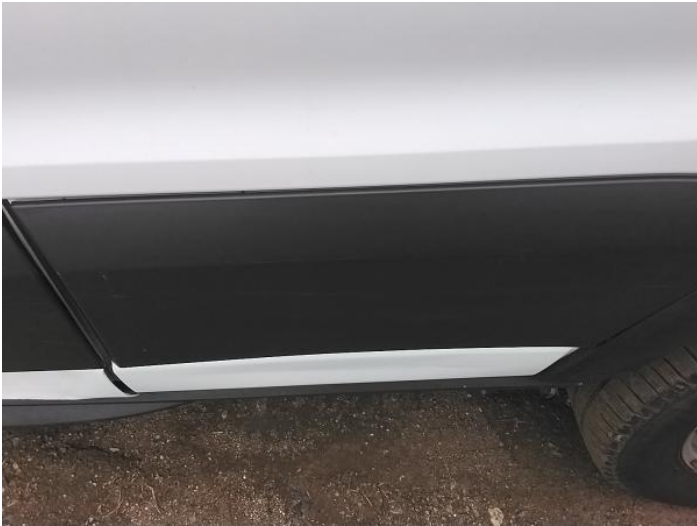
9: Qtr Panel Moulding ns Scuffed (Unpainted) Over 100mm
