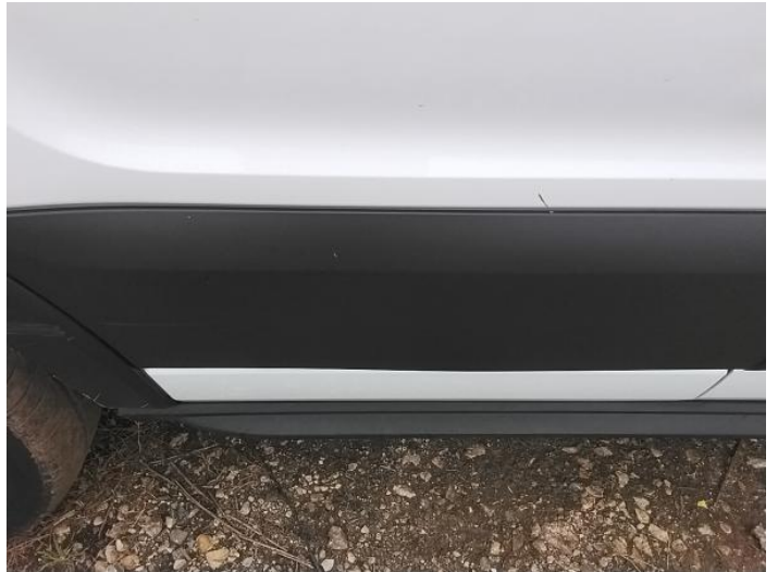
4: Door Moulding nsf Scuffed (Unpainted) Over 100mm
