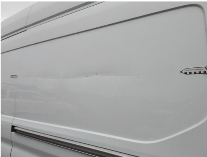
11: Qtr Panel nsr Dented With Paint Damage
