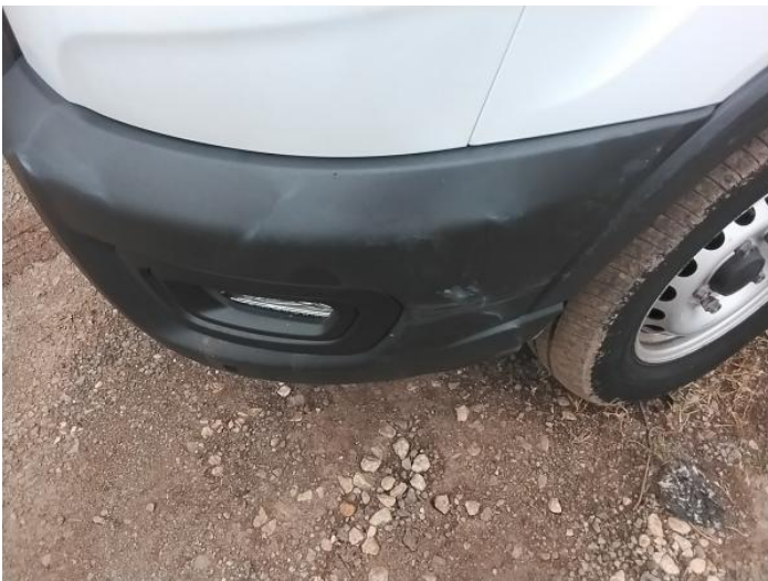
1: Bumper Front Scratched Over 100mm Thru Paint
