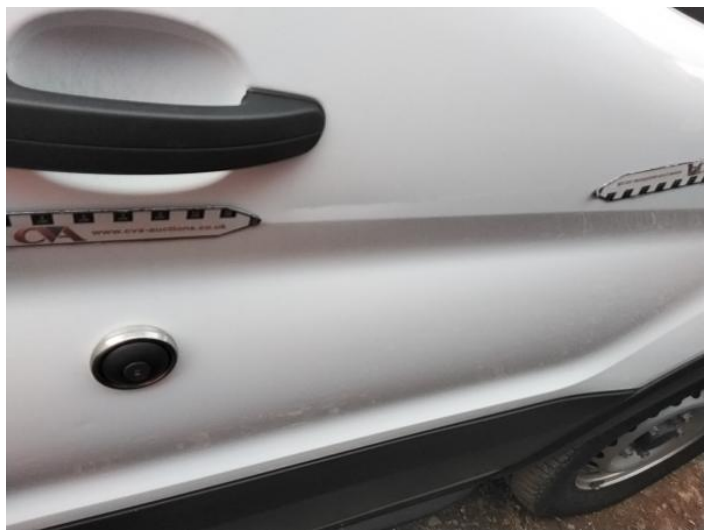
20: Door osf Dented With Paint Damage
