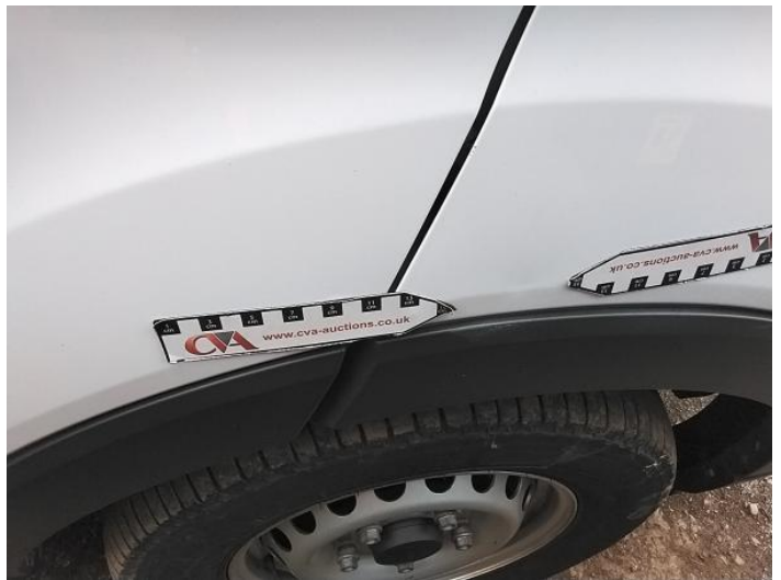
18: Wing osf Dented Over 30mm
