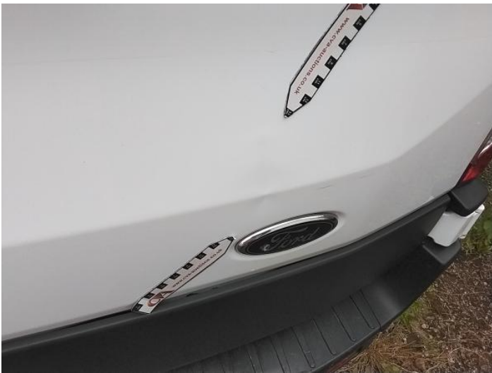
17: Door osr Dented Over 30mm
