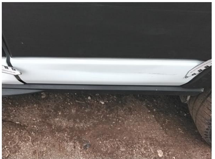
8: Qtr Panel nsr Dented With Paint Damage
