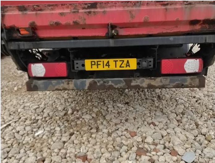
9: Bumper Rear Rusted Over 5mm
