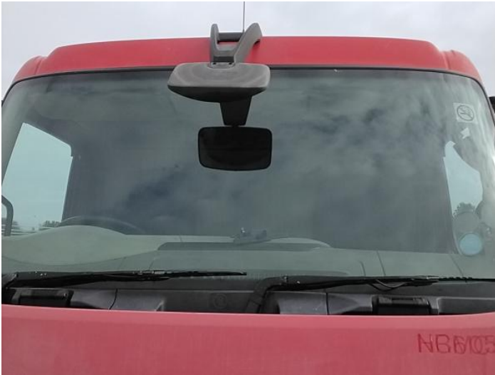
3: Screen Front Chipped Over 10mm
