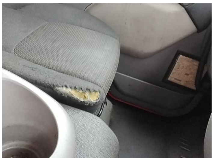
14: Seat Base Cover nsf Holed Over 3mm
