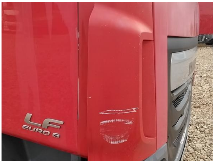
1: Wing osf Scratched Over 25mm Thru Paint
