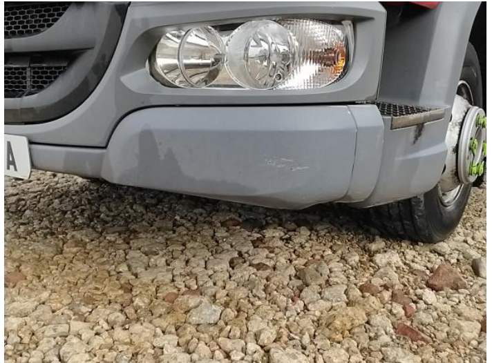
4: Bumper Front Moulding Scratched (Painted) UpTo 25mm Thru Paint
