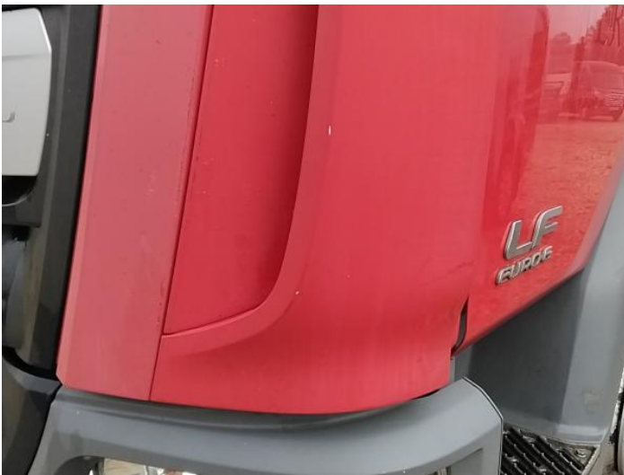
5: Wing nsf Scratched UpTo 25mm Thru Paint
