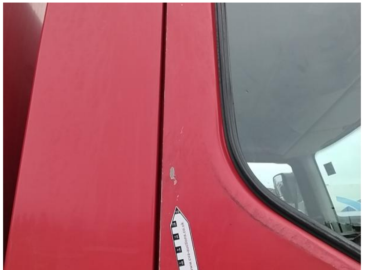
12: Door osf Scratched UpTo 25mm Thru Paint
