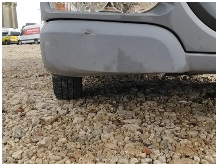
2: Bumper Front Moulding Scratched (Painted) UpTo 25mm Thru Paint
