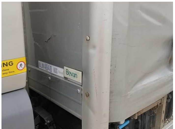
8: C Post ns Dented Between 10mm + 30mm
