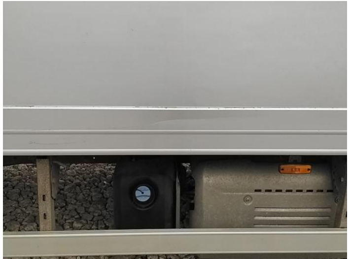
10: Qtr Panel osr Dented Between 10mm + 30mm
