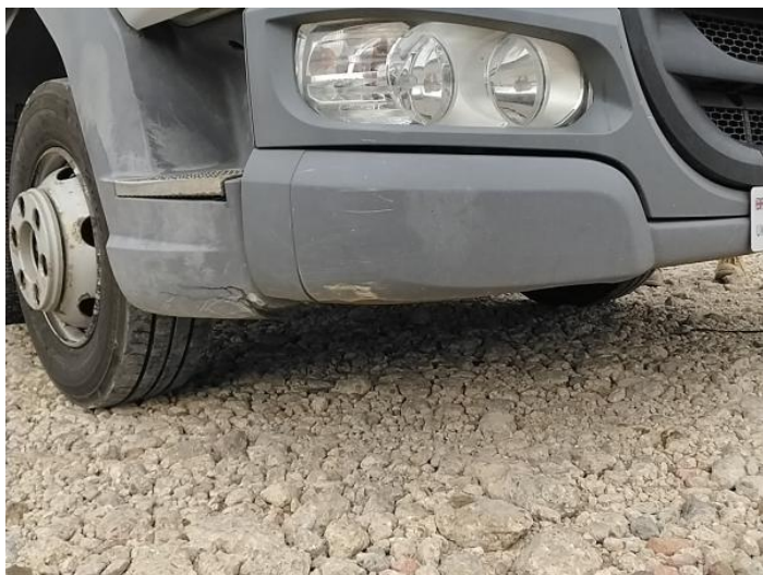
1: Bumper Front Moulding Scratched (Painted) Over 25mm Thru Paint
