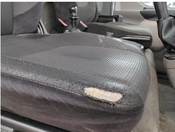
13: Seat Base Cover osf Holed Over 3mm
