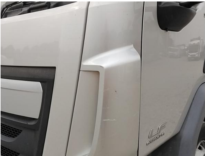
5: Wing nsf Scratched Over 25mm Thru Paint
