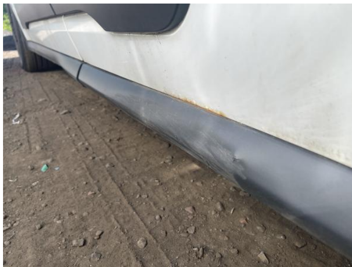
2: Door nsr Rusted Over 5mm
