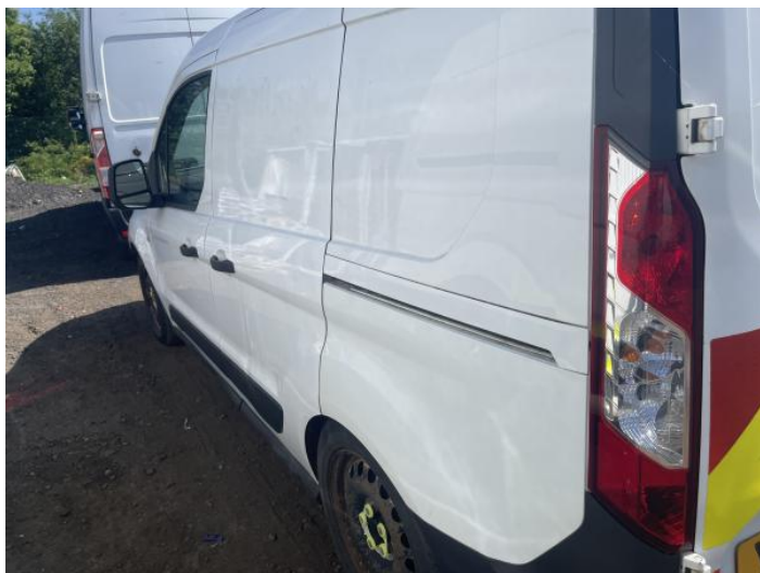
1: Qtr Panel nsr Dented Over 30mm
