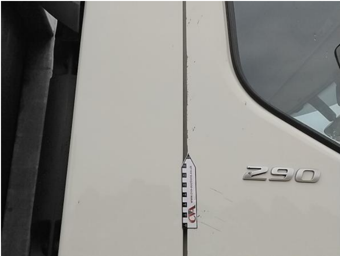
9: Door osf Chipped Edge Chip
