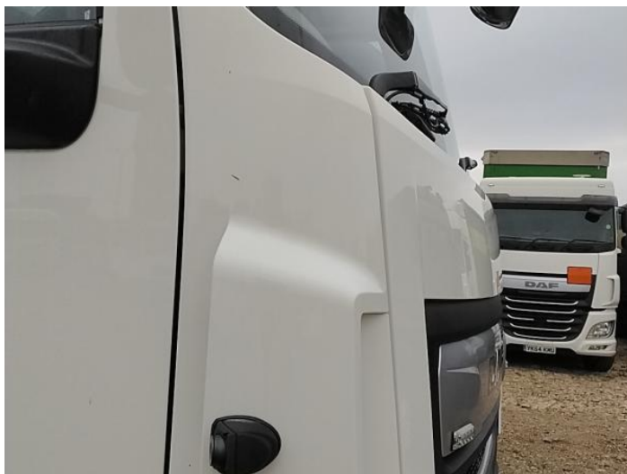
1: Wing osf Scratched UpTo 25mm Thru Paint
