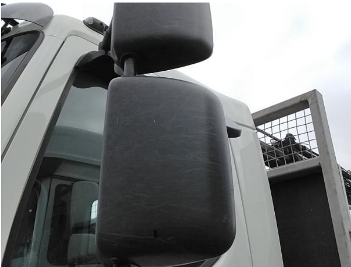
5: Door Mirror Assy nsf Scuffed (Unpainted) UpTo 100mm
