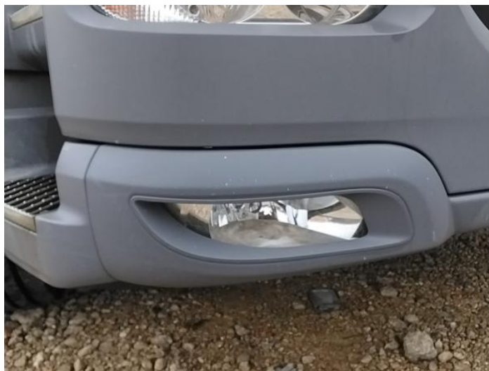
2: Bumper Front Chipped Multiple Chips
