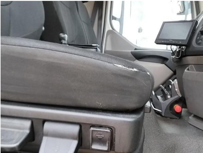
11: Seat Base Cover osf Holed Over 3mm
