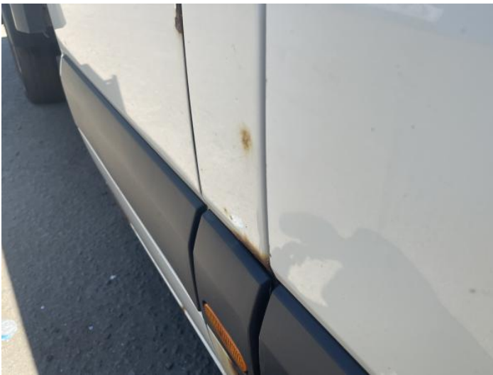
5: B Post os Rusted Over 5mm
