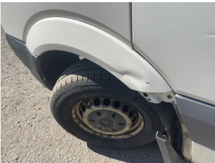
13: Wing nsf Dented With Paint Damage
