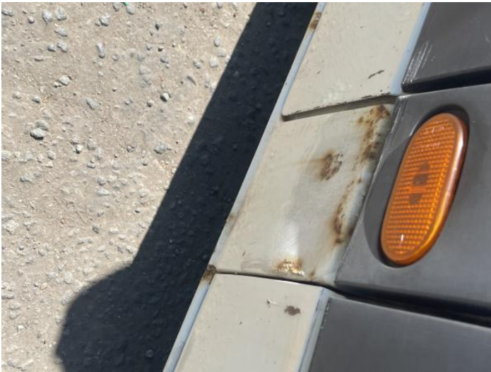
11: B Post ns Rusted Over 5mm
