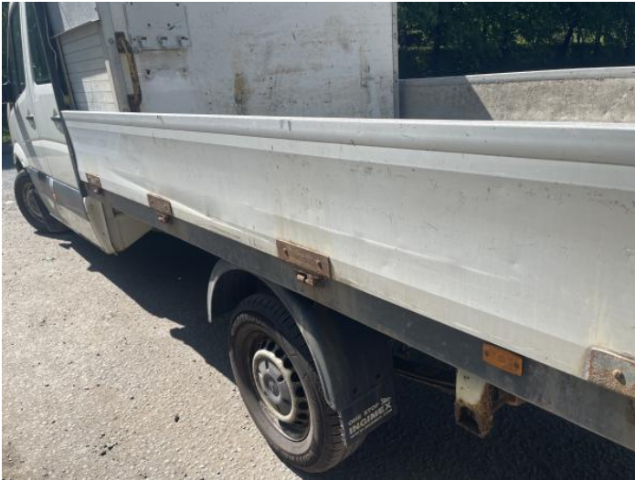
9: Qtr Panel nsr Dented With Paint Damage
