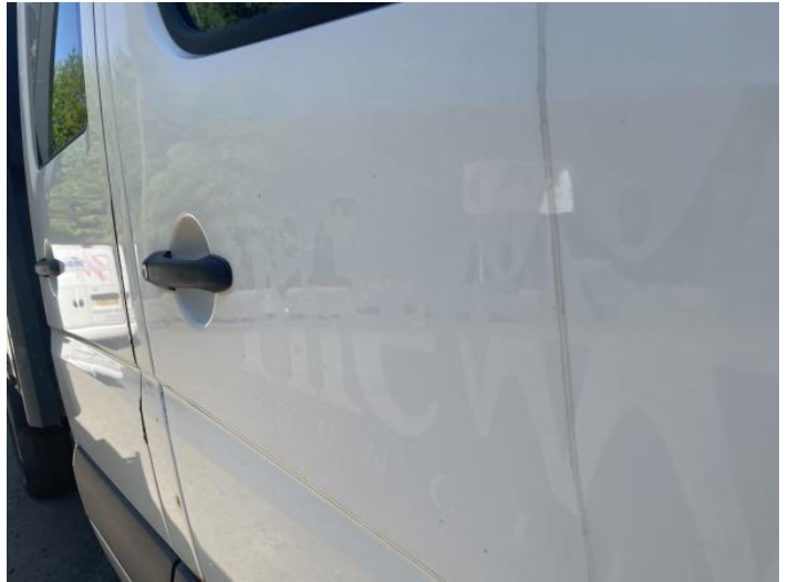
4: Door osf Dented With Paint Damage
