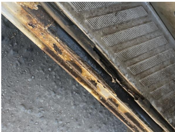
1: Sill os Rusted Over 5mm
