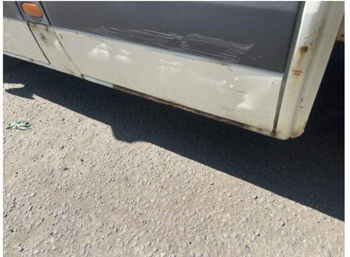
10: Door nsr Dented With Paint Damage
