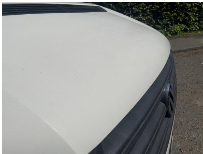
2: Bonnet Dented Over 30mm
