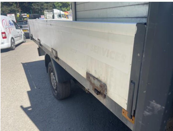
7: Qtr Panel osr Dented With Paint Damage
