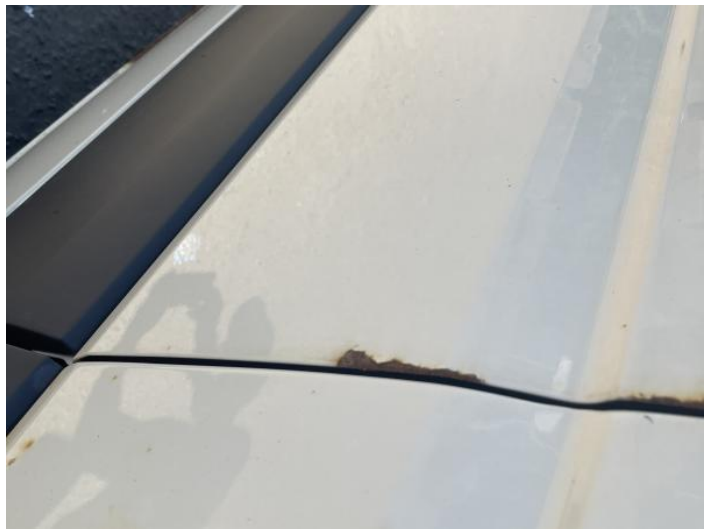
6: Door osr Rusted Over 5mm
