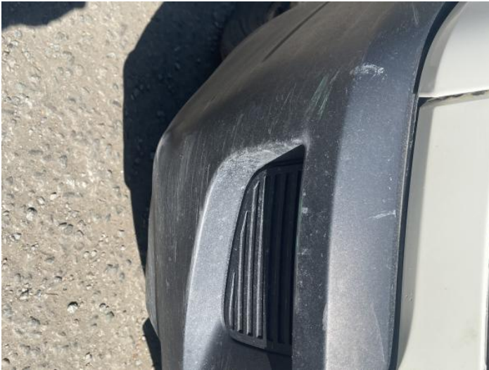
3: Bumper Front Moulding Scuffed (Unpainted) Over 100mm
