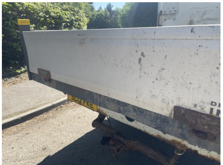
8: Tailgate Dented With Paint Damage
