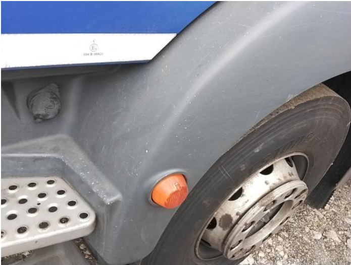
3: Wing nsf Chipped Multiple Chips
