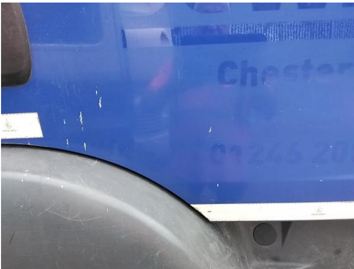
5: Door osf Scratched Over 25mm Thru Paint
