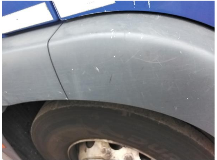
4: Wing osf Chipped Multiple Chips
