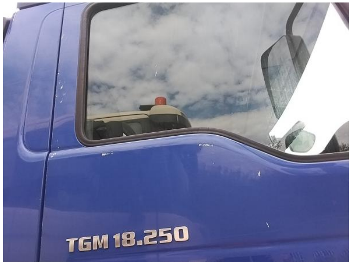
6: Door osf Scratched Over 25mm Thru Paint
