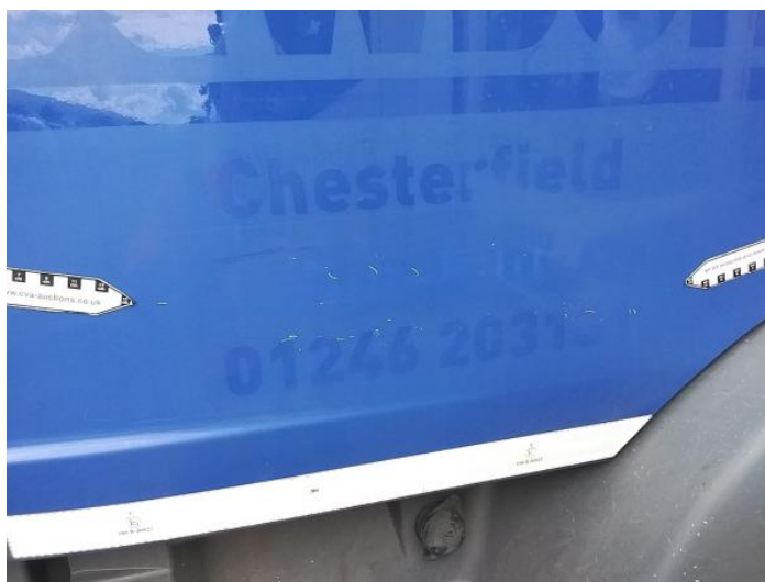
2: Door nsf Scratched Over 25mm Thru Paint
