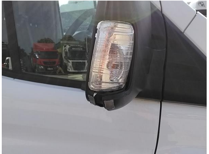
28: Door Mirror Assy osf Broken Replace
