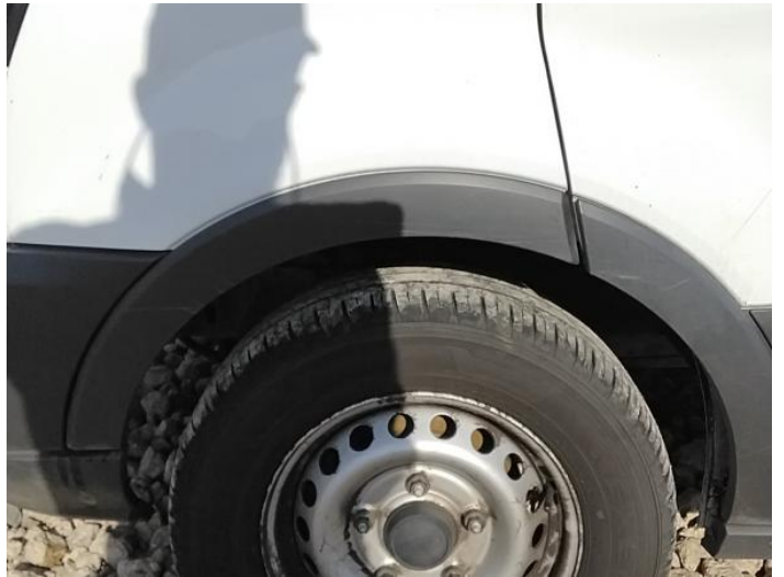
6: Moulding nsf Wing Scuffed (Unpainted) Over 100mm
