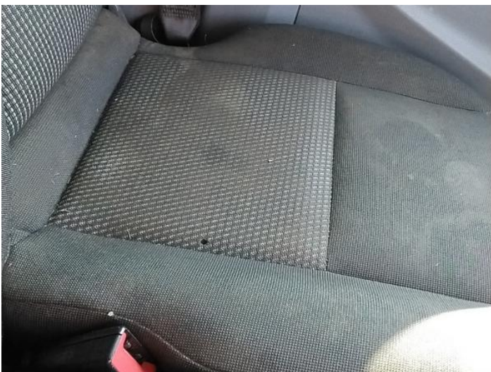
31: Seat Base Cover nsf Burn Over 3mm
