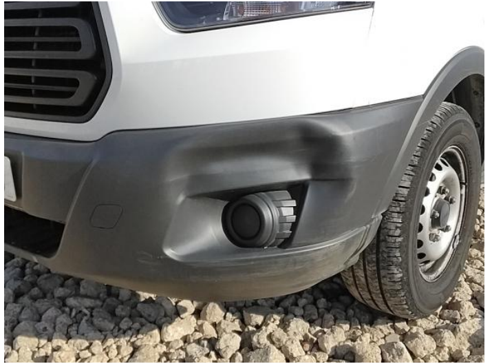
4: Bumper Front Dented Over 30mm
