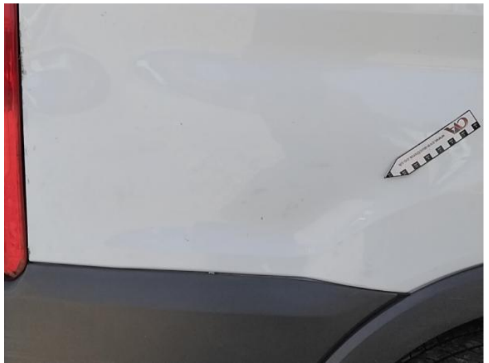
24: Qtr Panel osr Dented Between 10mm + 30mm
