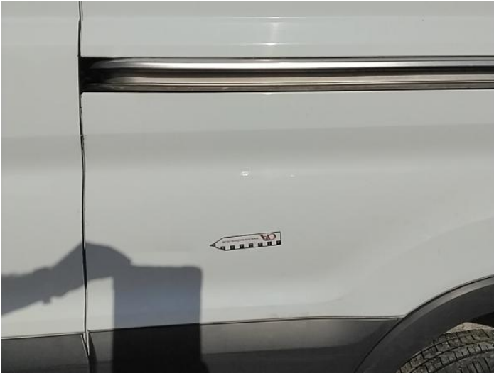
15: Qtr Panel nsr Dented Between 10mm + 30mm
