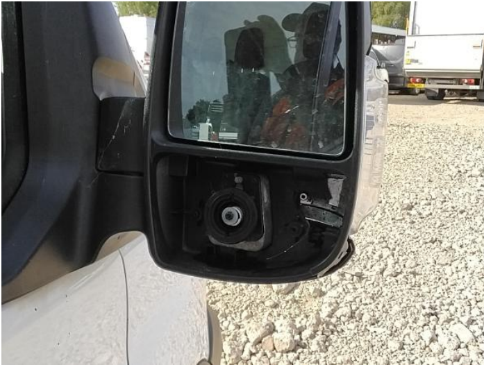
27: Door Mirror Glass os Missing Replace
