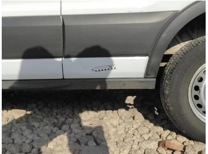
16: Qtr Panel nsr Dented With Paint Damage
