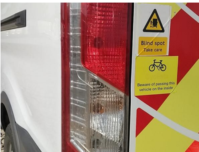
19: Lamp nsr Broken Replace
