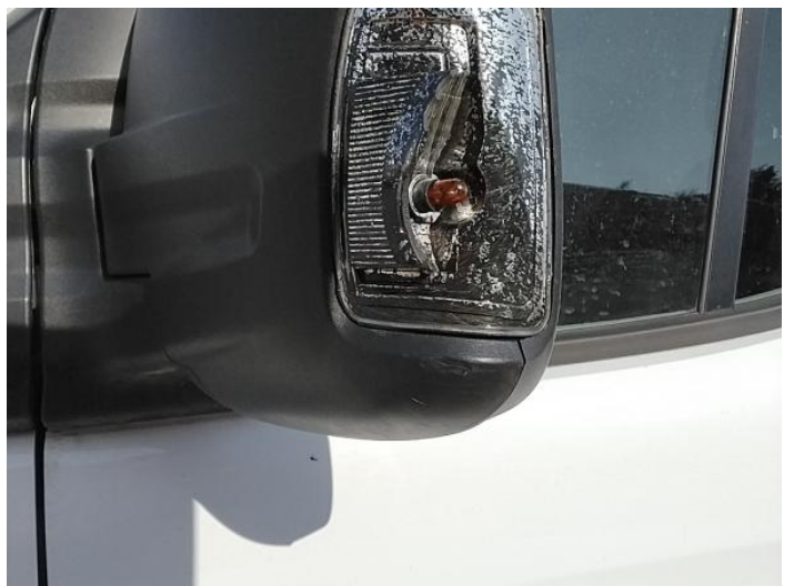
8: Flasher Side Repeater ns Broken Replace
