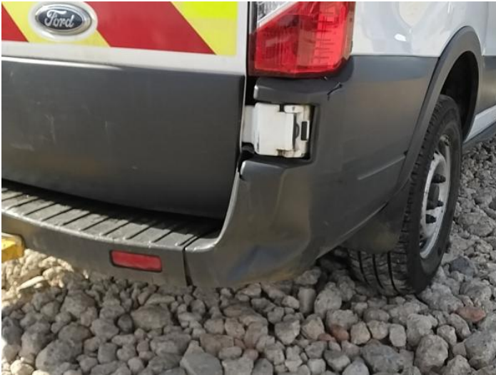
21: Bumper Rear Moulding Broken Replace
