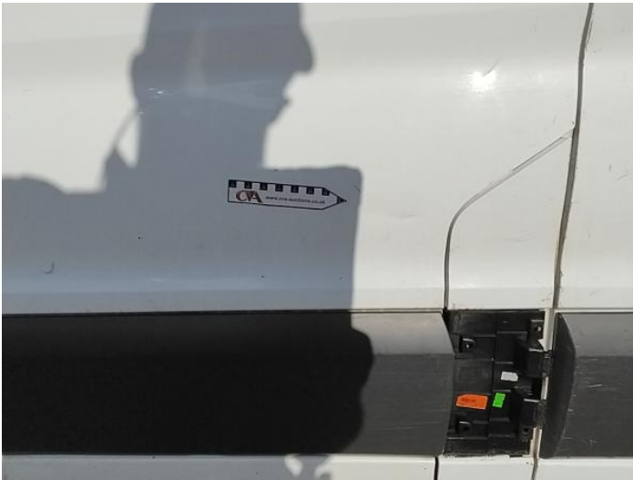
11: Door nsf Dented Between 10mm + 30mm
