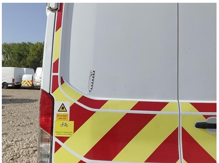
20: Door nsr Dented With Paint Damage
