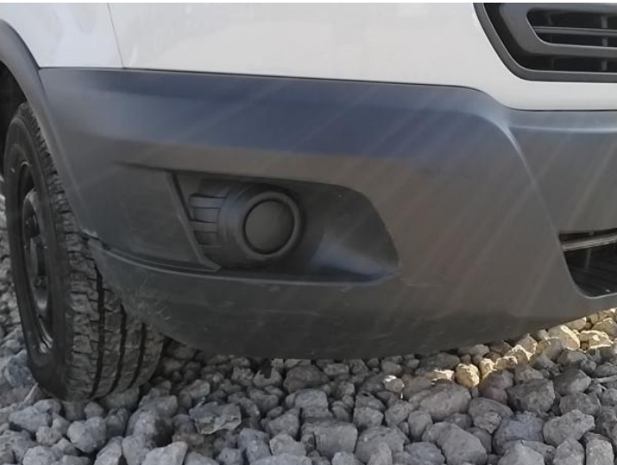
1: Bumper Front Moulding Scuffed (Unpainted) Over 100mm
