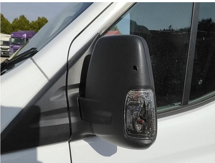
7: Door Mirror Assy nsf Broken Replace
