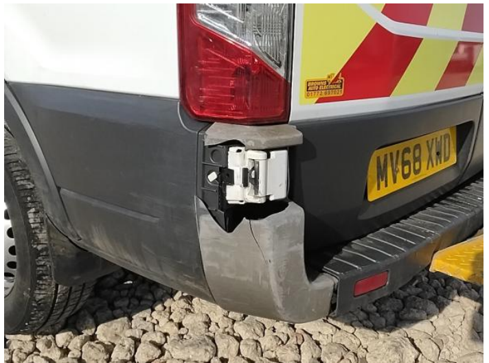
18: Bumper Rear Moulding Broken Replace
