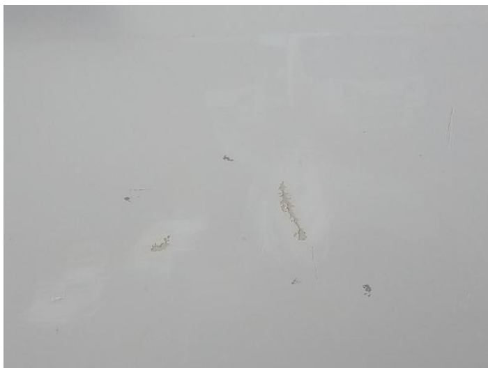
1: Panel Front Scratched Over 25mm Thru Paint
