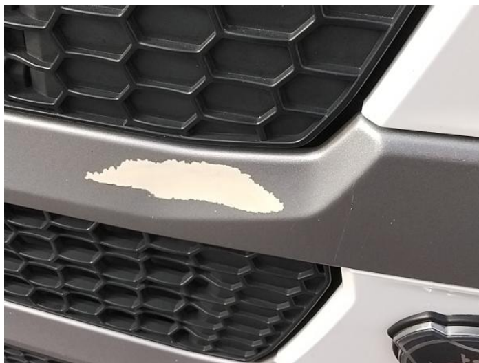
2: Panel Front Scratched Over 25mm Thru Paint
