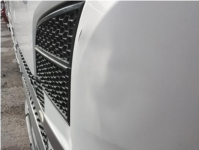
3: Bumper Front Dented Over 30mm
