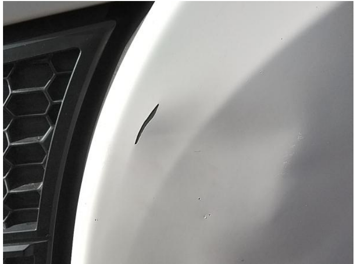
4: Panel Front Cracked Replace
