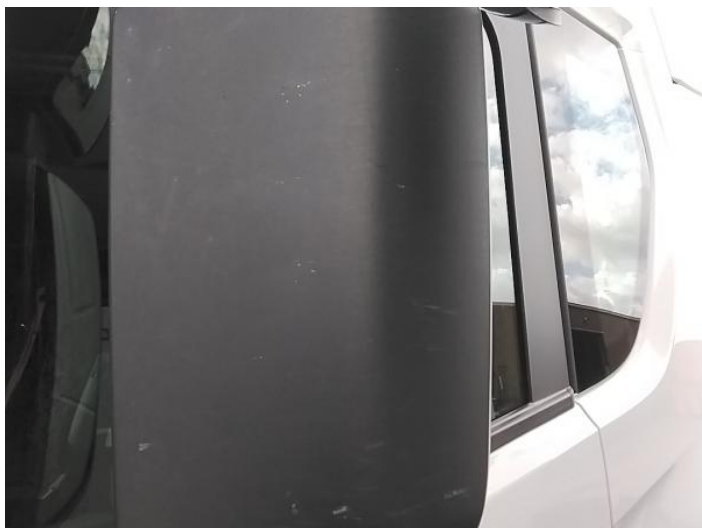
1: Door Mirror Assy nsf Scuffed (Unpainted) Over 100mm
