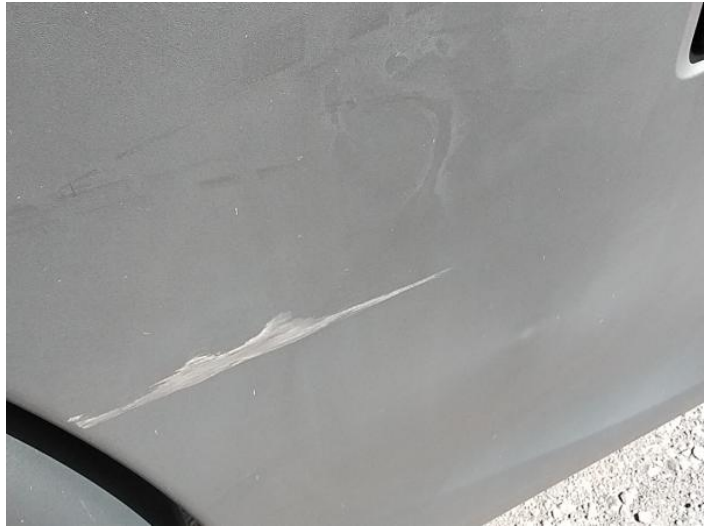
4: Sill Panel Trim os Scuffed (Unpainted) Over 100mm
