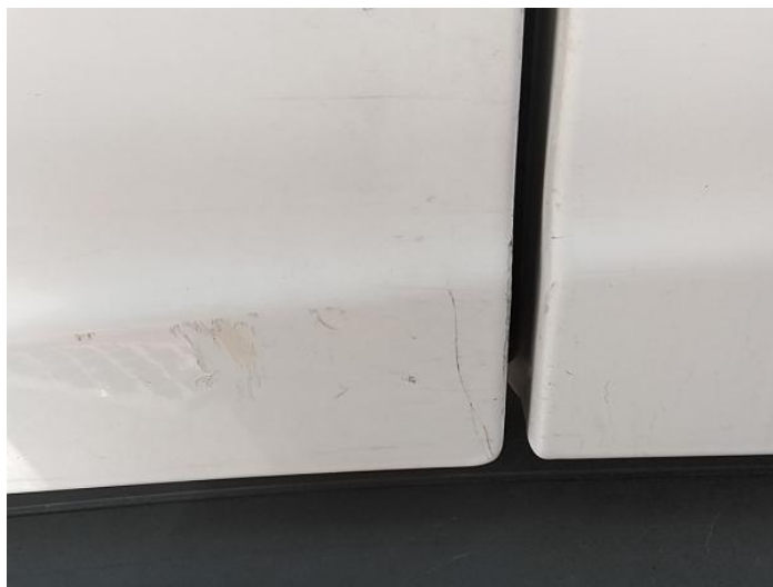
2: Door nsf Chipped Over 5mm
