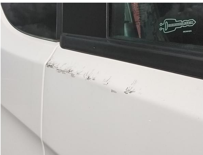
7: Door osf Scratched Over 25mm Not Thru Paint
