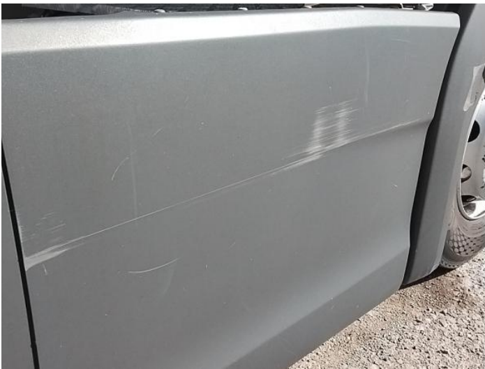
5: Sill Panel Trim os Scuffed (Unpainted) Over 100mm
