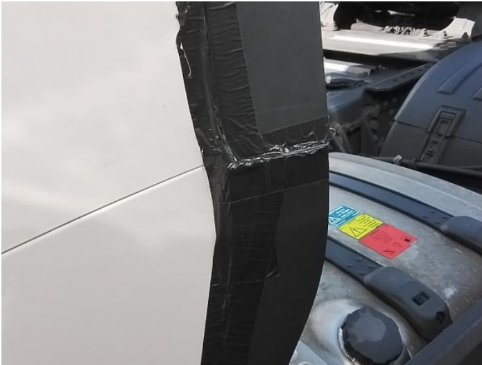
3: Panel Front Poor Previous Repair Rippled Up To 30%
