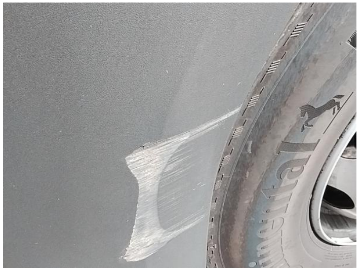
6: Wheel Trim osf Scratched Over 50mm
