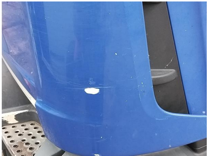
6: Bonnet Scratched Over 25mm Thru Paint
