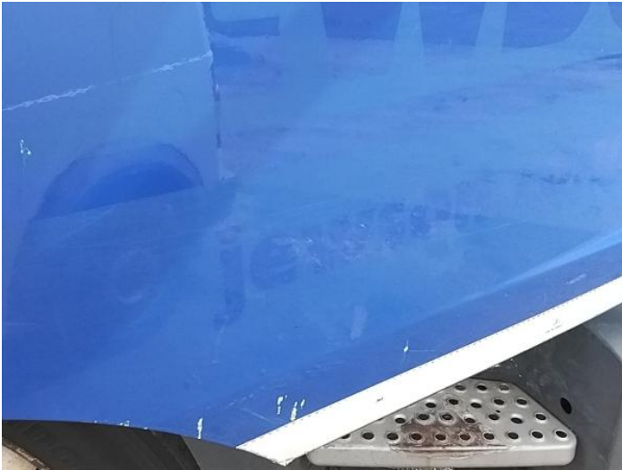
3: Door osf Chipped Multiple Chips
