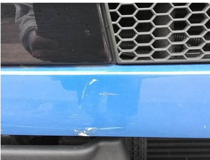
7: Grille Front Scratched (Painted) Over 25mm Thru Paint
