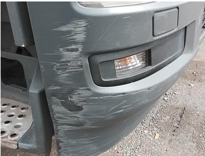
5: Bumper Front Moulding Scuffed (Unpainted) Over 100mm
