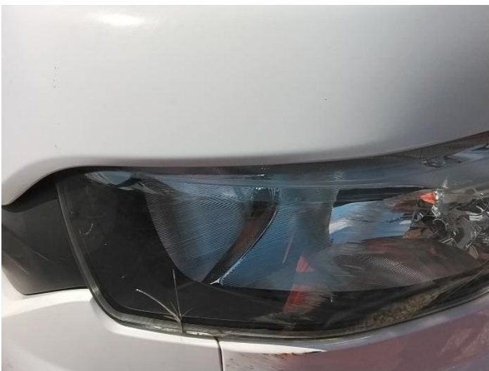
7: Headlamp ns Broken Replace
