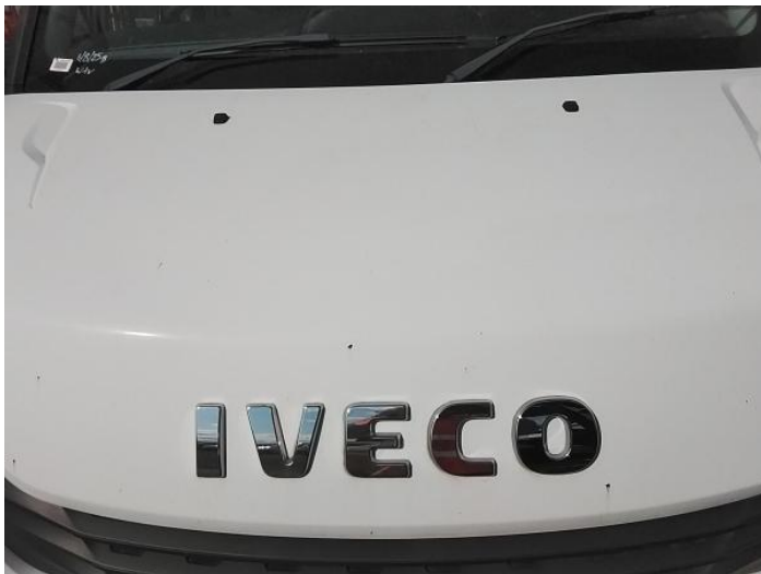
1: Bonnet Chipped Multiple Chips
