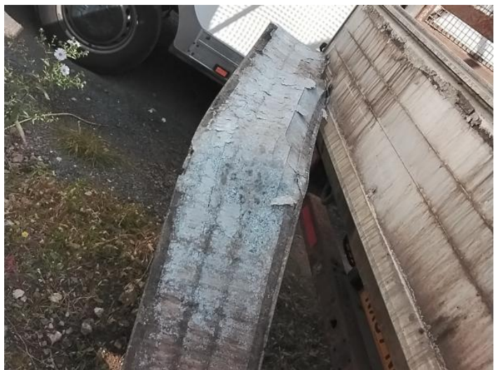
8: Tailgate Trim Panel Broken Replace
