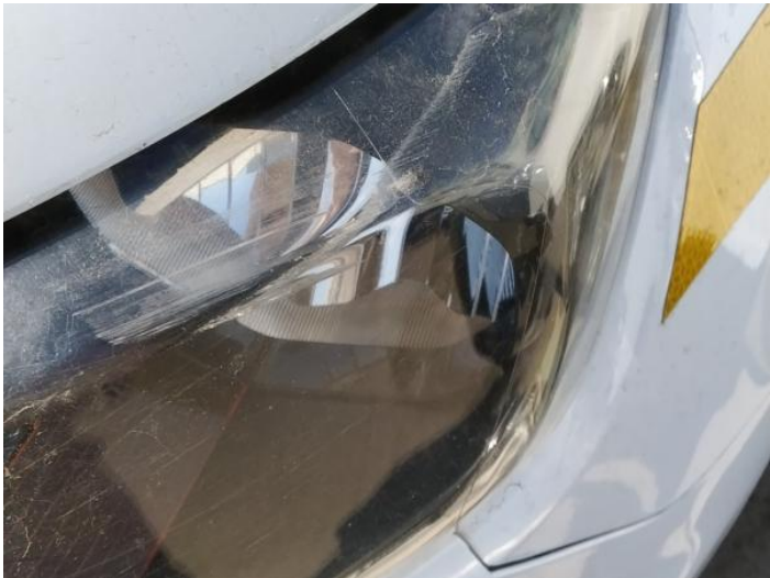
2: Lamp osr Broken Replace
