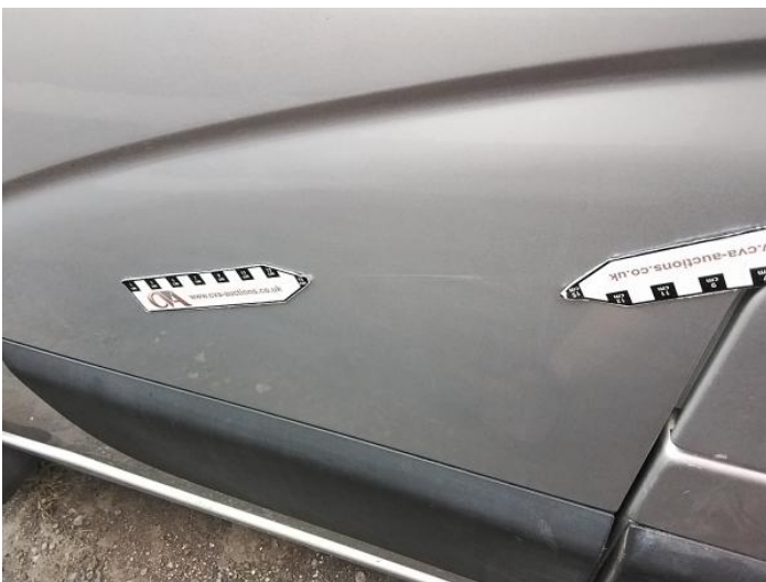
7: Door nsf Scratched Over 25mm Thru Paint
