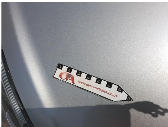
2: Bonnet Scratched Over 25mm Thru Paint
