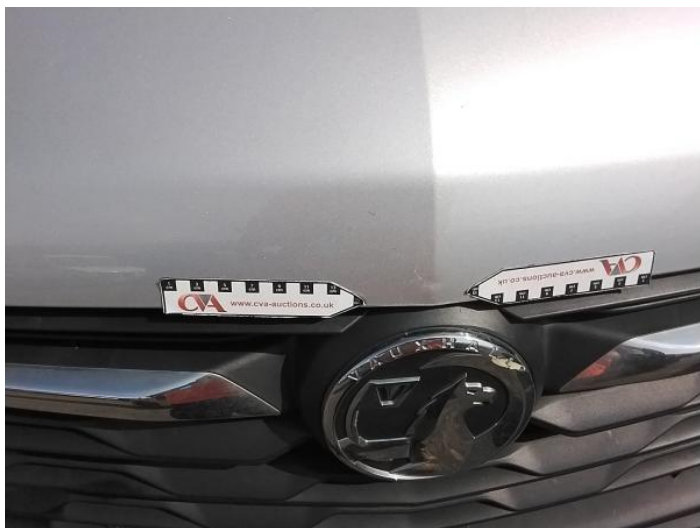
1: Bonnet Dented With Paint Damage
