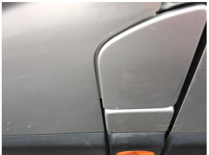
8: Fuel Flap Scratched Over 25mm Thru Paint
