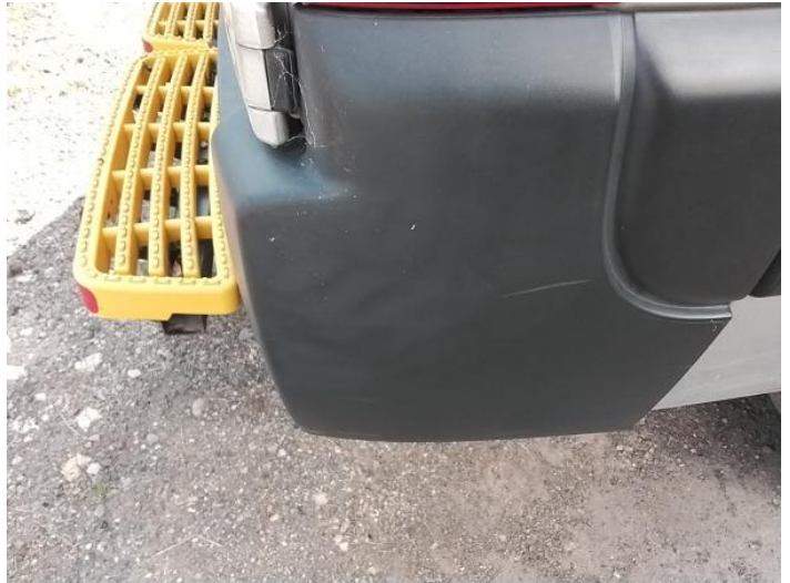
16: Bumper Rear Moulding Scuffed (Unpainted) UpTo 100mm
