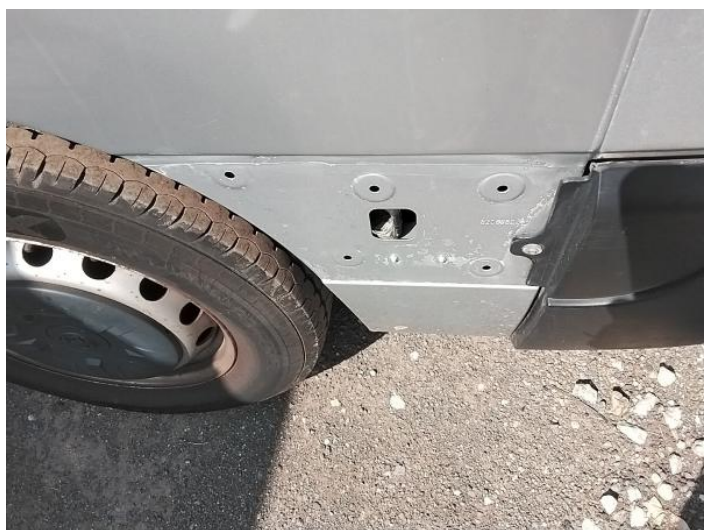
14: Qtr Panel Moulding ns Missing Replace
