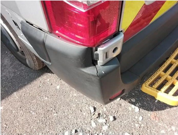
15: Bumper Rear Moulding Broken Replace
