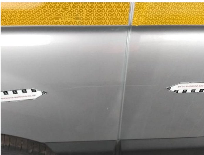
19: Qtr Panel osr Scratched Over 25mm Thru Paint
