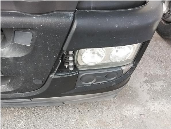
3: Bumper Front Moulding Missing Replace
