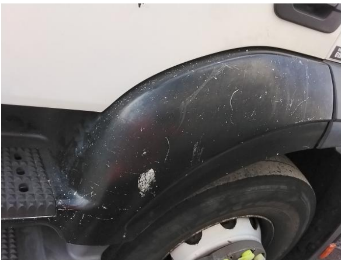
7: Wing nsf Scratched Over 25mm Thru Paint
