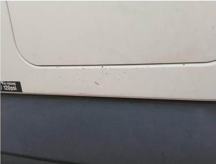
9: Qtr Panel nsr Chipped Multiple Chips
