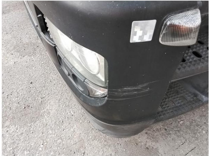
4: Bumper Front Scratched Over 100mm Thru Paint
