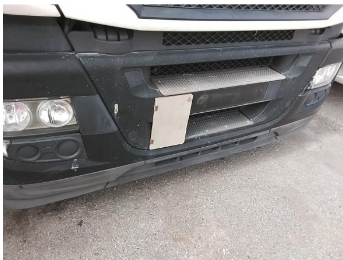
2: Bumper Front Chipped Multiple Chips
