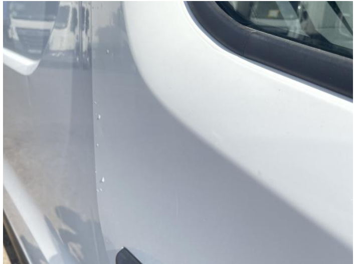
4: Door osf Dented With Paint Damage
