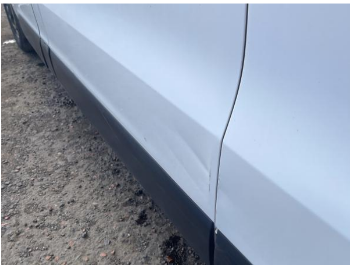
7: Door nsr Dented With Paint Damage
