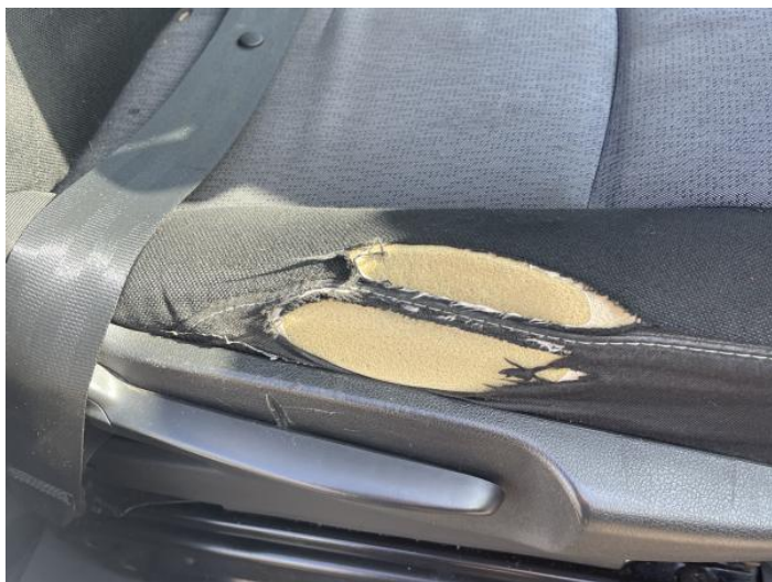
1: Seat Base Cover osf Torn Over 3mm
