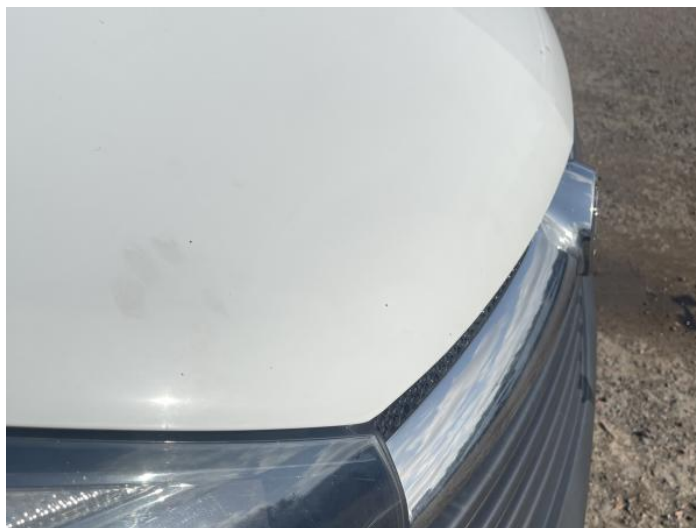
2: Bonnet Dented With Paint Damage
