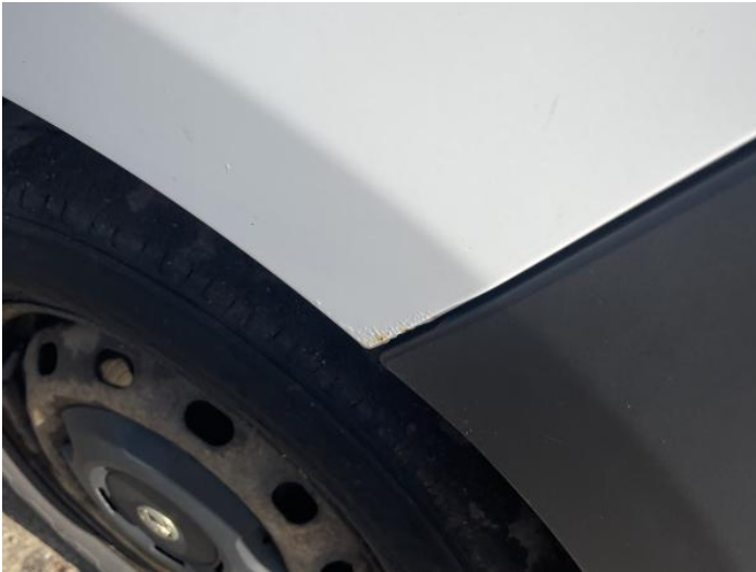
3: Wing osf Rusted Over 5mm
