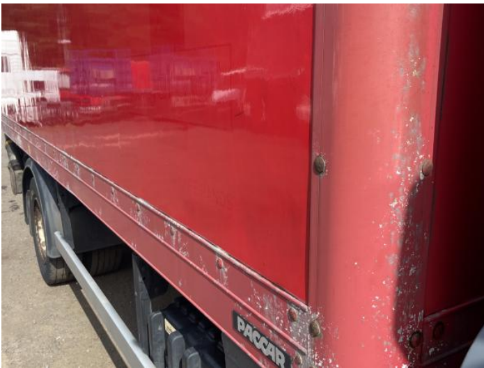
5: Qtr Panel osr Rusted Over 5mm
