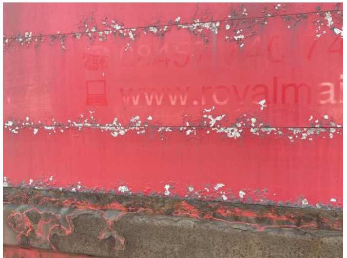
6: Tailgate Rusted Over 5mm
