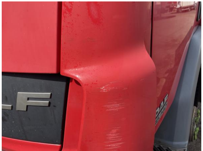
10: Wing nsf Scratched Over 25mm Thru Paint
