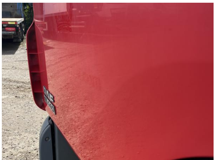
8: Door nsf Dented Over 30mm
