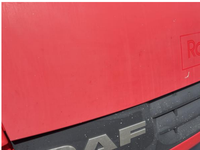
1: Bonnet Chipped Multiple Chips
