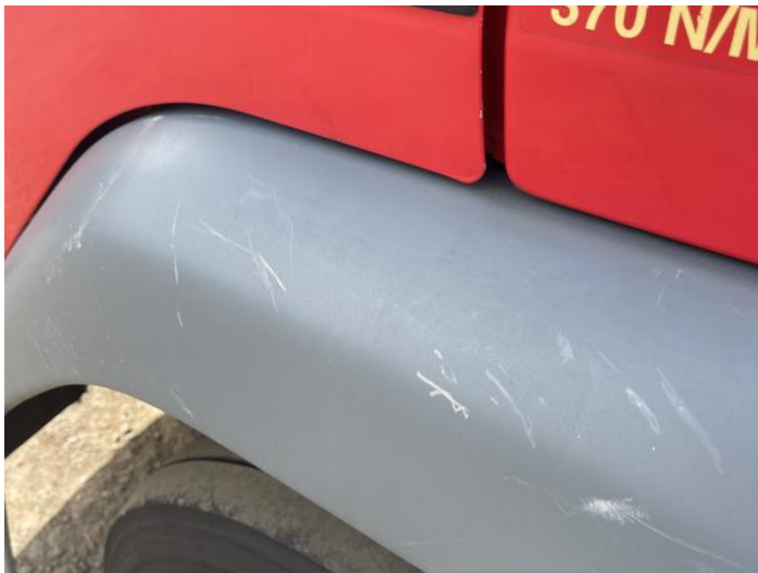
9: Door Moulding nsf Scuffed (Unpainted) Over 100mm
