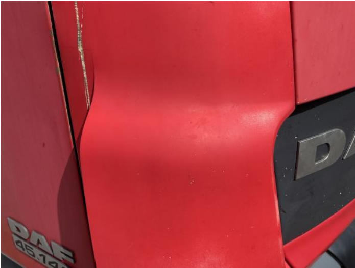
3: Wing nsf Cracked Replace
