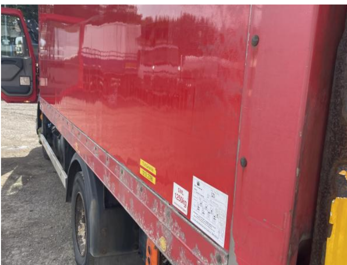
7: Qtr Panel nsr Rusted Over 5mm
