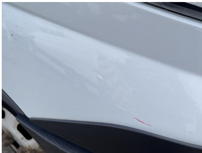
2: Wing of Scratched Over 25mm Thru Paint
