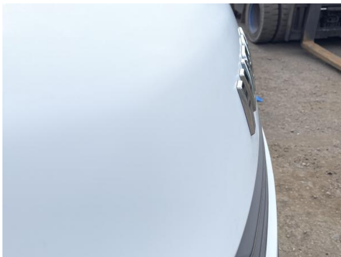
1: Bonnet Dented Over 30mm
