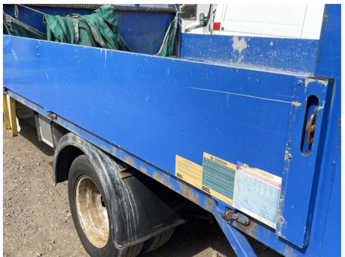
6: Qtr Panel nsr Dented Over 30mm
