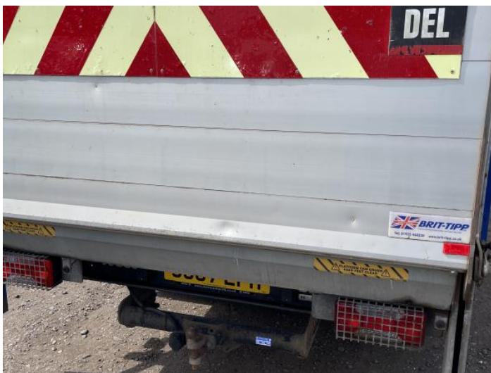
5: Tailgate Dented Over 30mm
