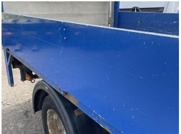
4: Qtr Panel osr Dented With Paint Damage
