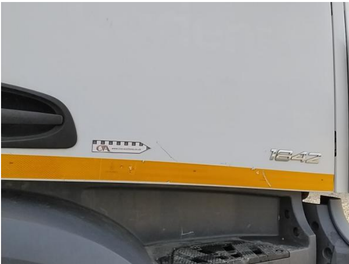
7: Door osf Scratched UpTo 25mm Thru Paint
