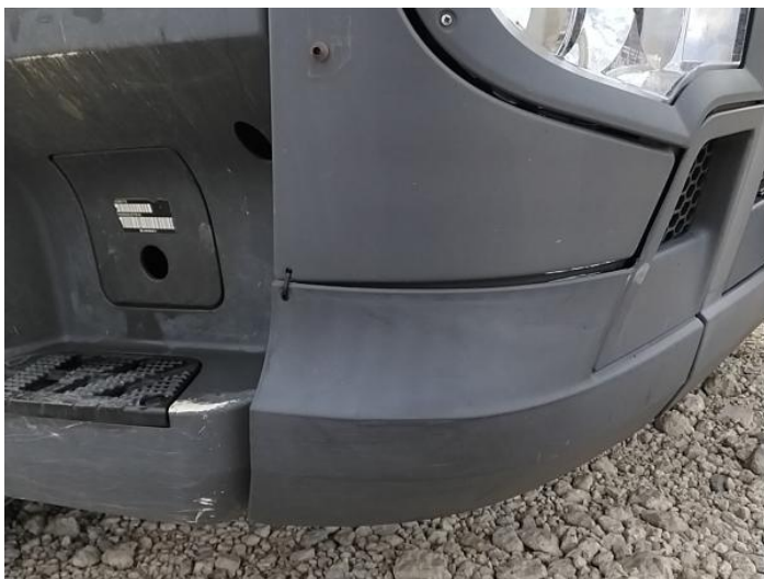
1: Bumper Front Moulding Broken Replace
