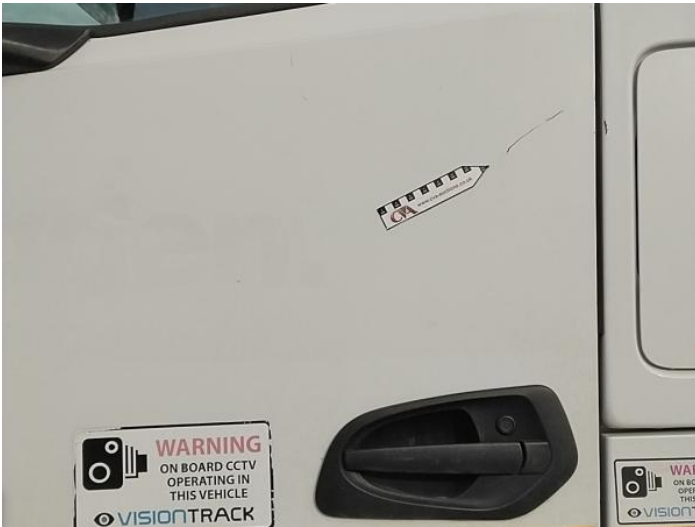
5: Door nsf Scratched UpTo 25mm Thru Paint
