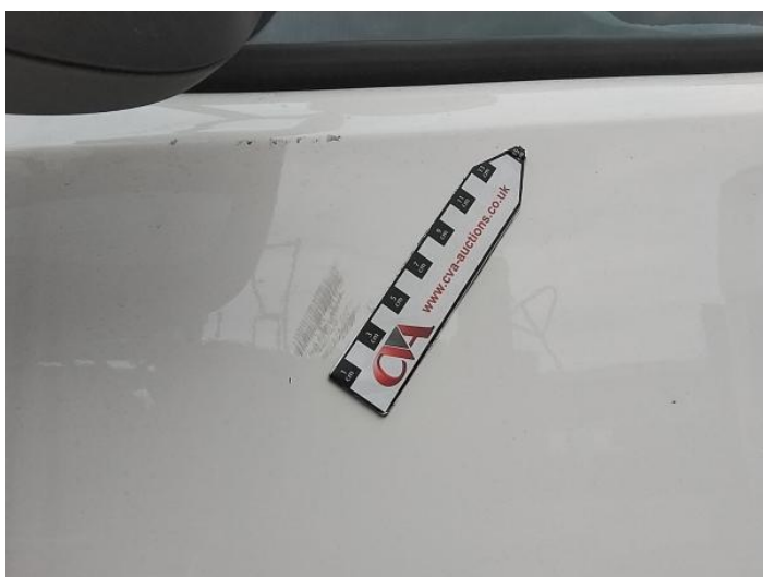
5: Door nsf Scratched Over 25mm Thru Paint
