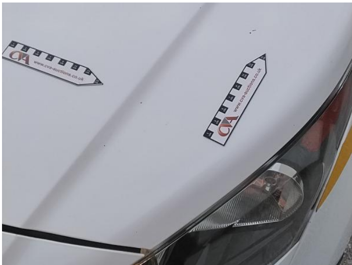
1: Bonnet Chipped Multiple Chips
