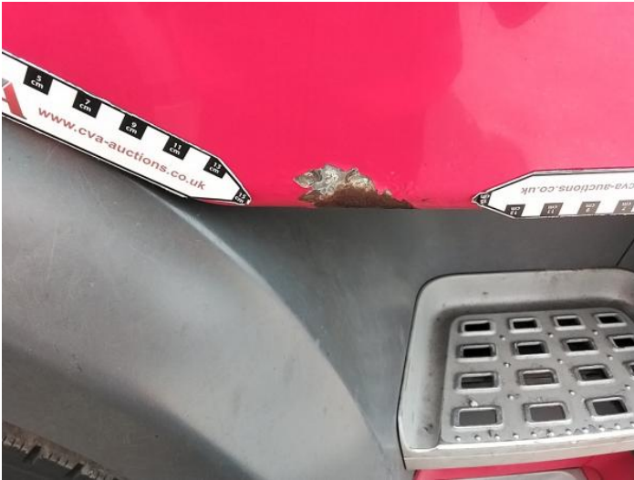
9: Door osf Rusted Over 5mm
