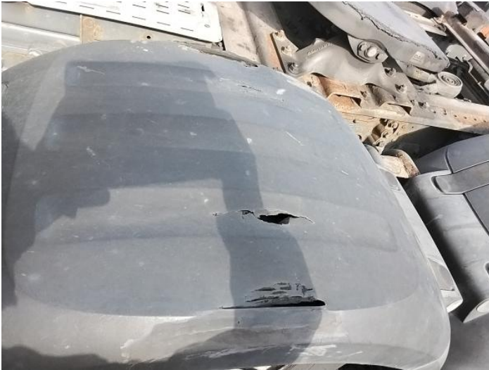
3: Qtr Panel Moulding ns Broken Replace
