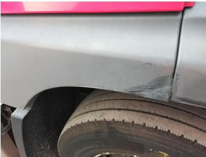
11: Qtr Panel Moulding os Scuffed (Unpainted) UpTo 100mm
