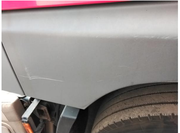
10: Qtr Panel Moulding os Scuffed (Unpainted) Over 100mm
