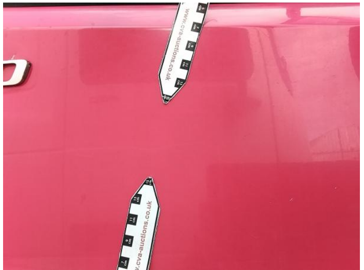
6: Door osf Dented Over 30mm
