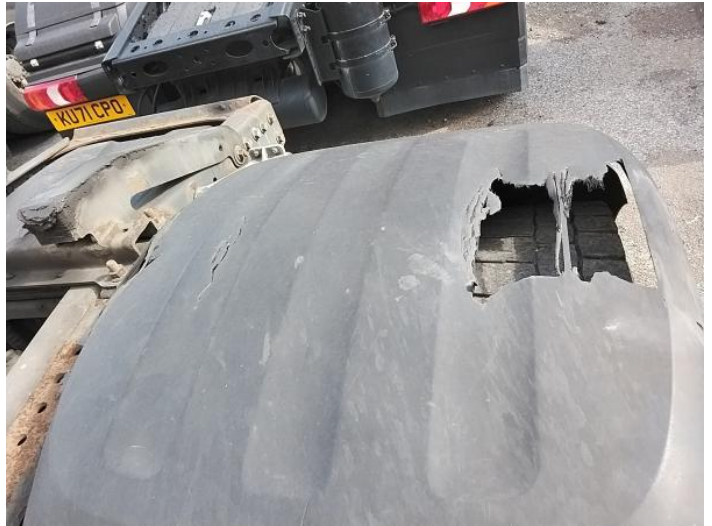
4: Qtr Panel Moulding ns Broken Replace
