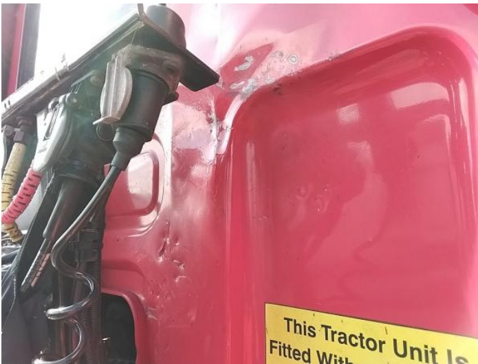
5: Panel Rear Dented With Paint Damage
