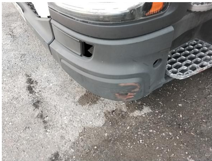
2: Bumper Front Scratched Over 100mm Thru Paint
