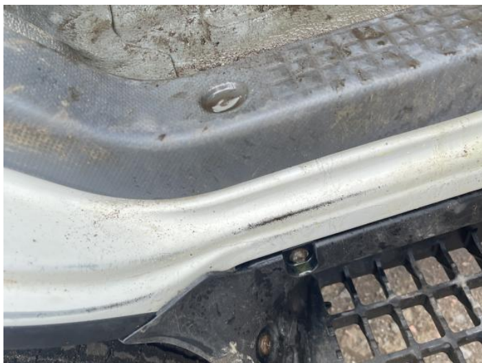
1: Sill os Rusted Over 5mm
