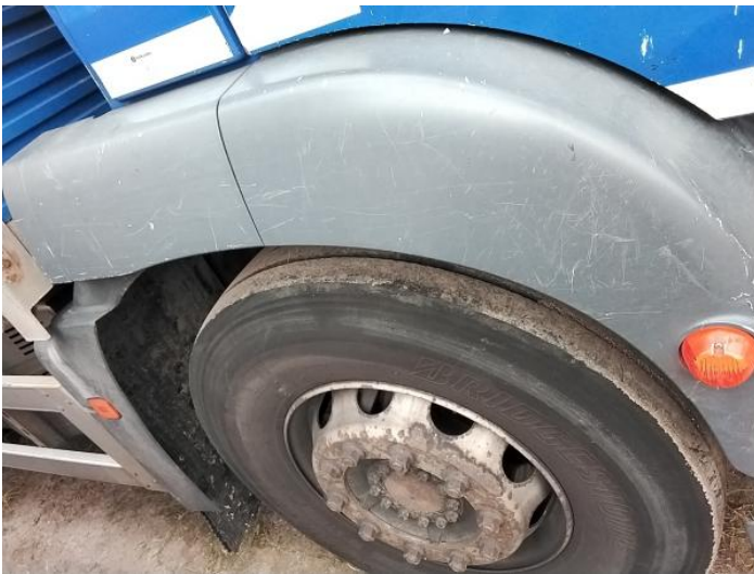
5: Qtr Panel Moulding os Scuffed (Unpainted) Over 100mm
