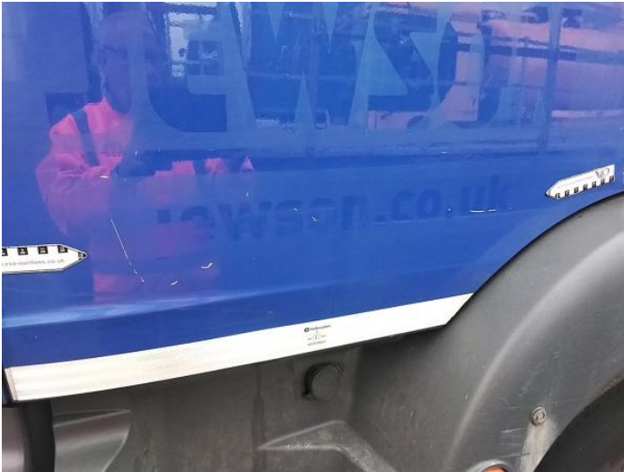
3: Door nsf Scratched Over 25mm Thru Paint
