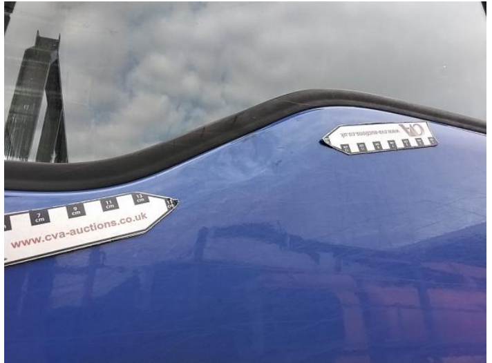
4: Door nsf Dented Over 30mm
