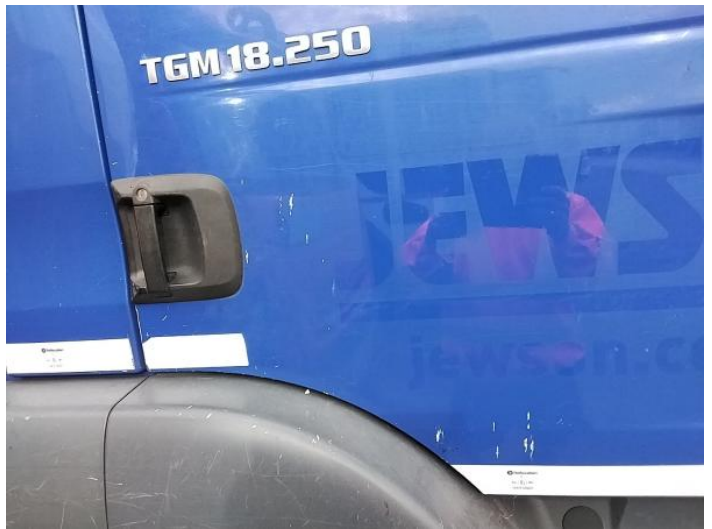
6: Door osf Scratched Over 25mm Thru Paint
