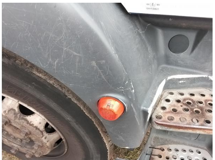
8: Wing osf Cracked Replace
