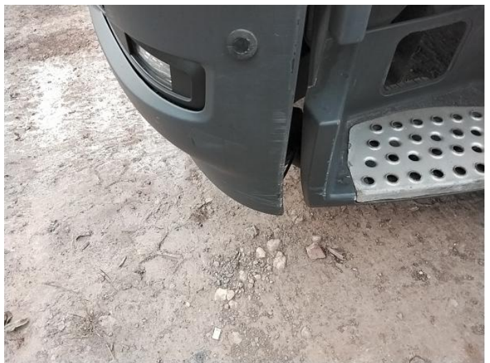
2: Bumper Front Scratched Over 100mm Thru Paint
