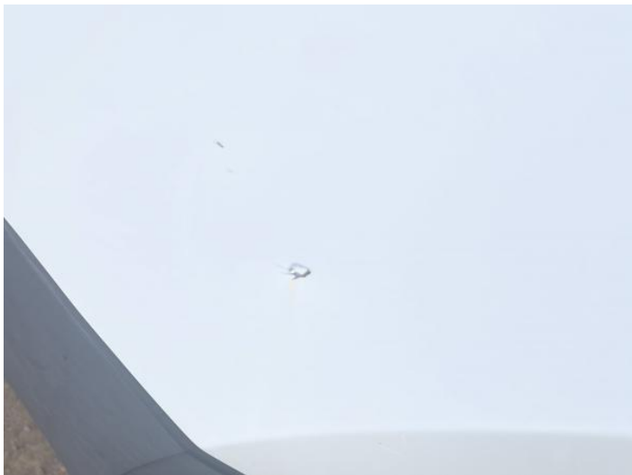
9: Wing nsf Dented With Paint Damage
