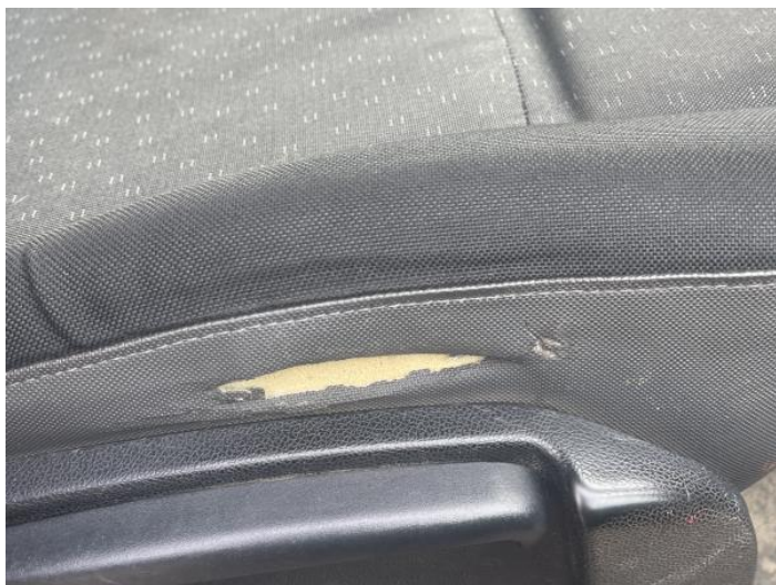
1: Seat Base Cover osf Torn Over 3mm
