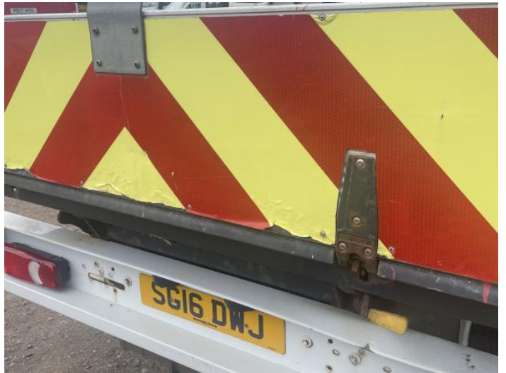
6: Tailgate Rusted Over 5mm
