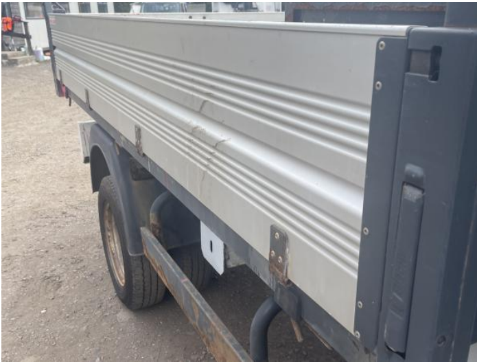
5: Qtr Panel osr Dented With Paint Damage
