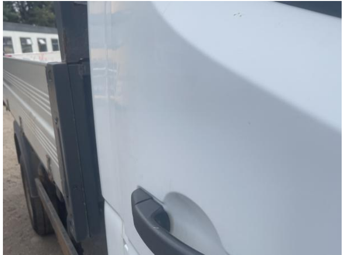
4: Door osf Dented Over 2 UpTo 10mm
