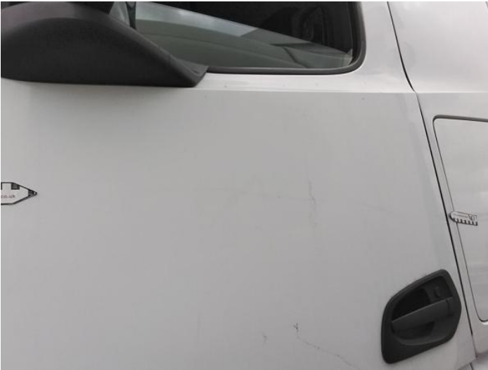
3: Door nsf Scratched Over 25mm Not Thru Paint
