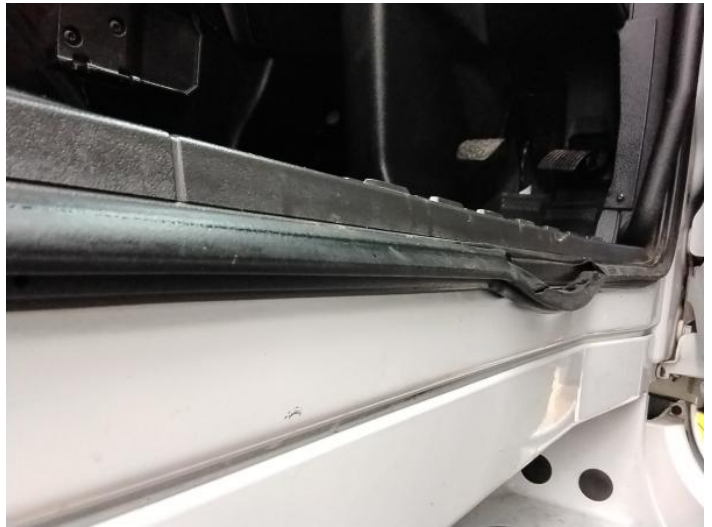
6: Aperture Seal osf Broken Replace
