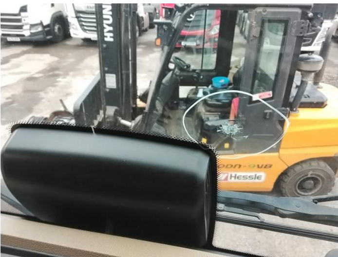
7: Screen Front Chipped Over 10mm
