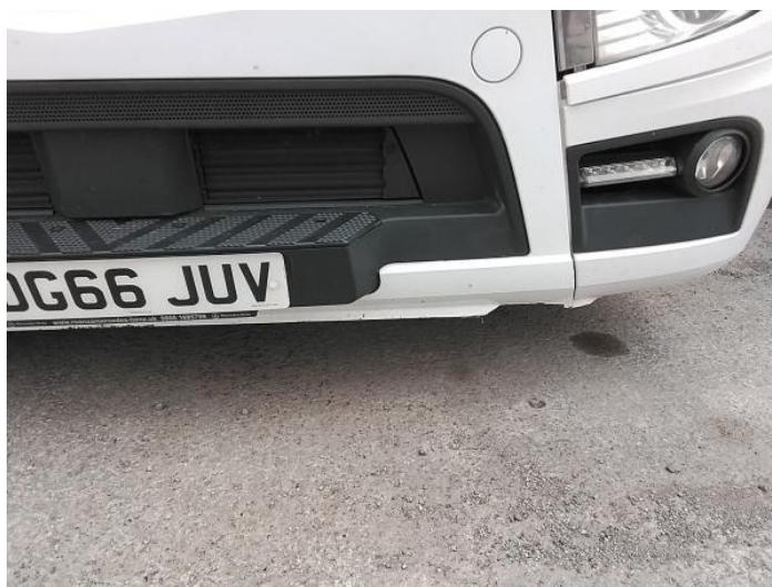
2: Bumper Front Cracked Over 25mm
