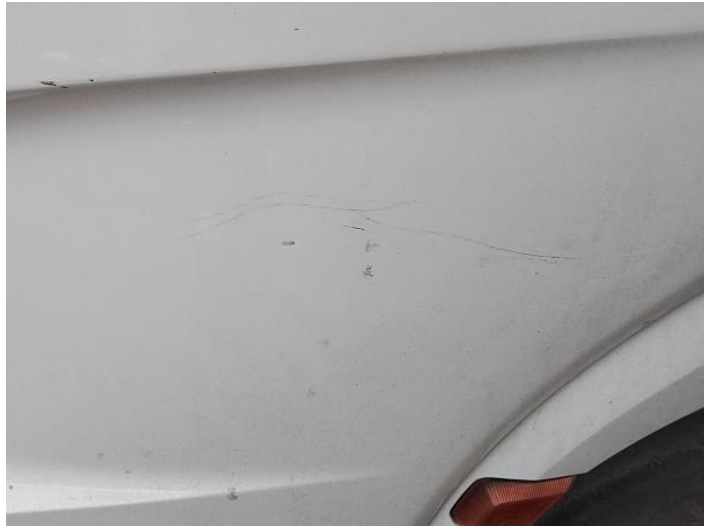
4: Door Moulding nsf Scratched (Painted) Over 25mm Thru Paint
