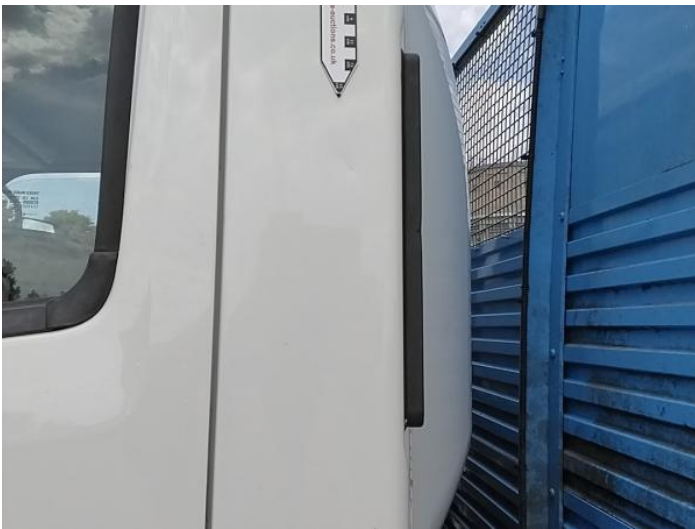
5: B Post ns Dented Over 2 UpTo 10mm
