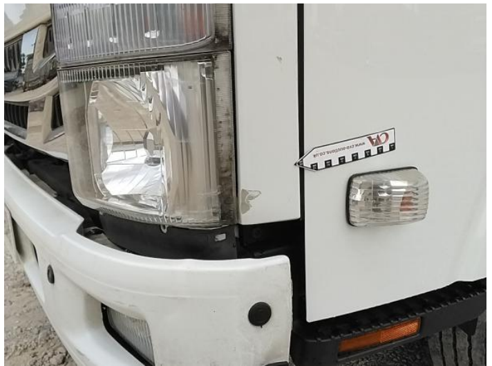
6: Wing nsf Scratched UpTo 25mm Thru Paint
