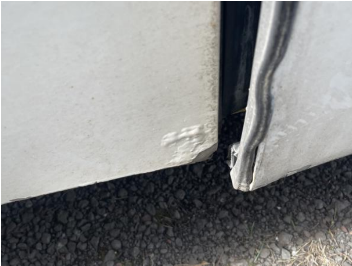
3: Qtr Panel osr Rusted Over 5mm
