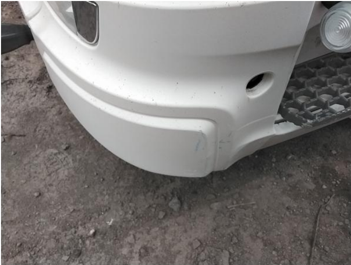
3: Bumper Front Scratched Over 25mm Not Thru Paint
