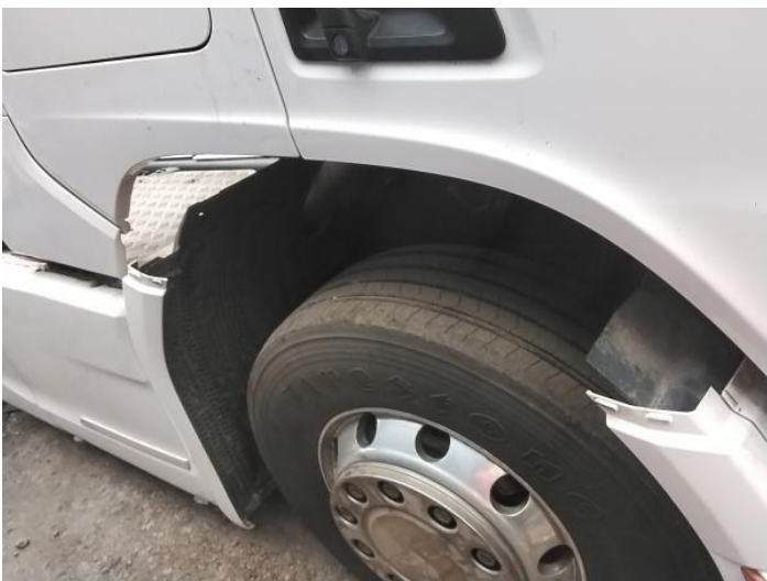
7: Wing nsf Missing Replace
