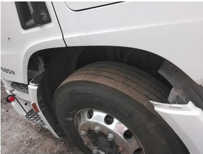
1: Wing nsf Missing Replace
