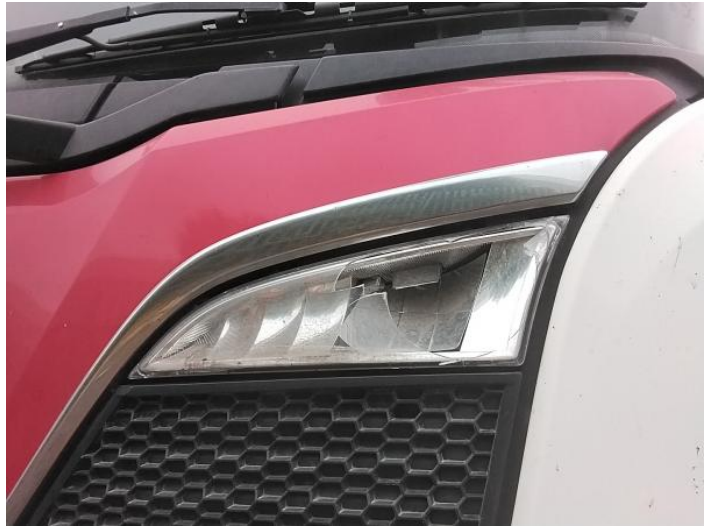
4: Fogdriving Lamp nsf Broken Replace
