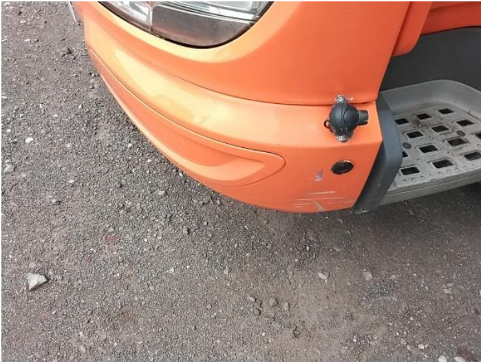
3: Bumper Front Dented With Paint Damage
