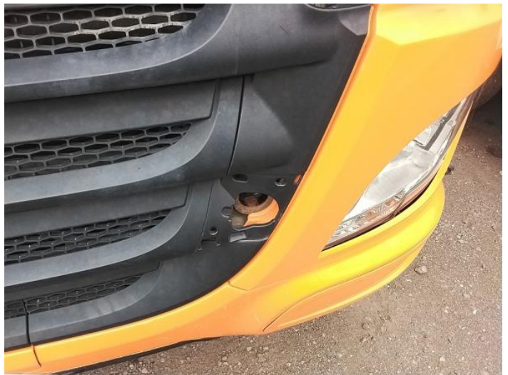
2: Bumper Front Moulding Missing Replace
