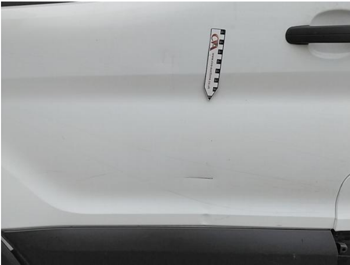
11: Door nsf Dented Between 10mm + 30mm
