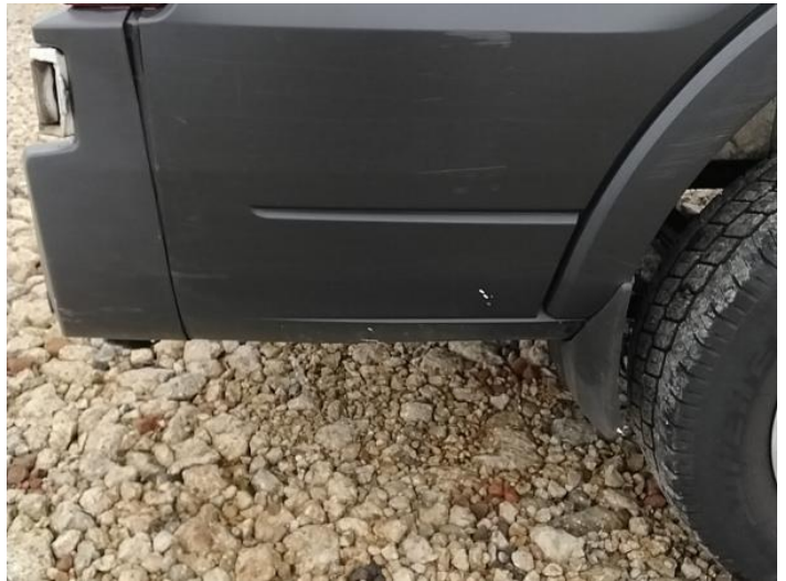
30: Qtr Panel Moulding os Scuffed (Unpainted) UpTo 100mm
