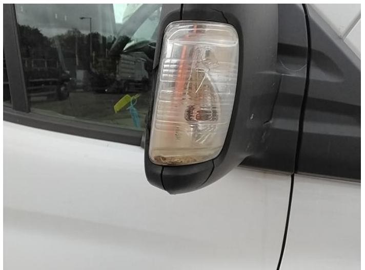
38: Flasher Side Repeater os Broken Replace
