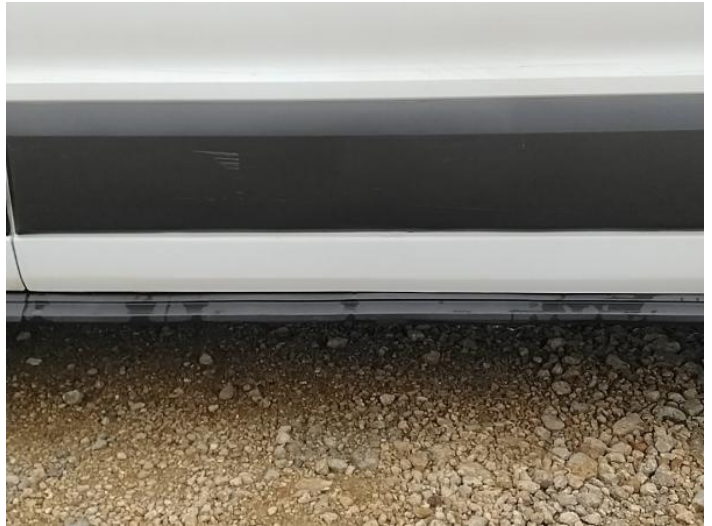
16: Door Moulding nsr Scuffed (Unpainted) Over 100mm
