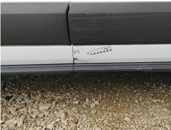
35: Door osf Dented With Paint Damage
