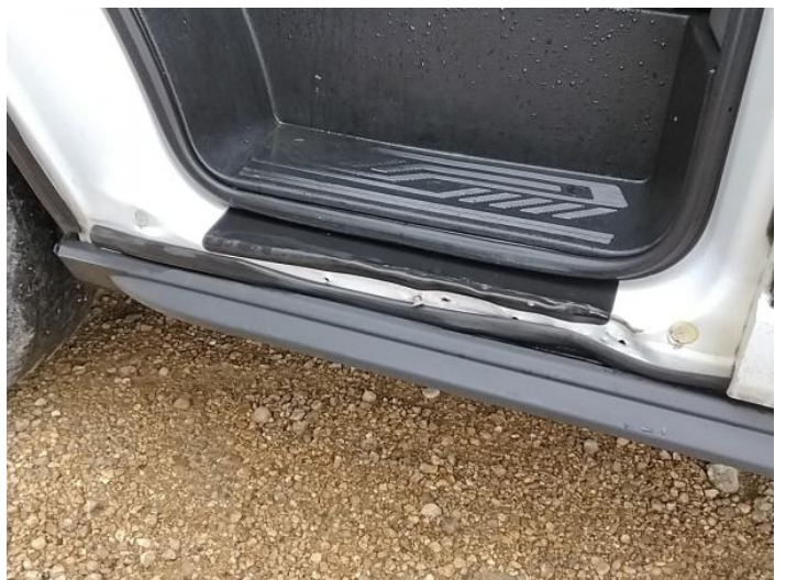
14: Sill ns Dented With Paint Damage
