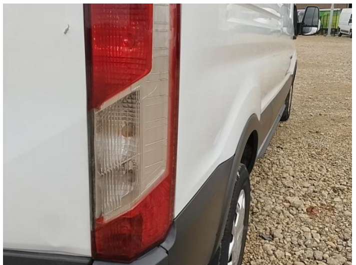
26: Lamp osr Broken Replace
