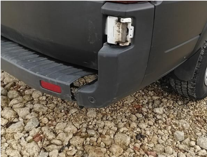
27: Bumper Rear Moulding Broken Replace
