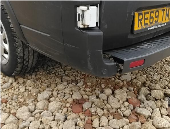
21: Bumper Rear Moulding Broken Replace
