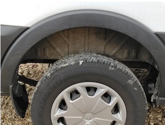
31: Qtr Panel Arch Extension os Scuffed (Unpainted) Over 100mm
