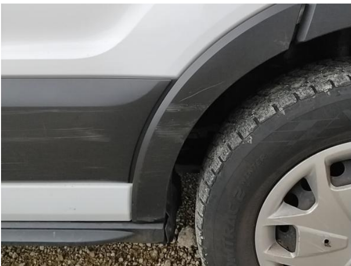
37: Moulding osf Wing Scuffed (Unpainted) UpTo 100mm
