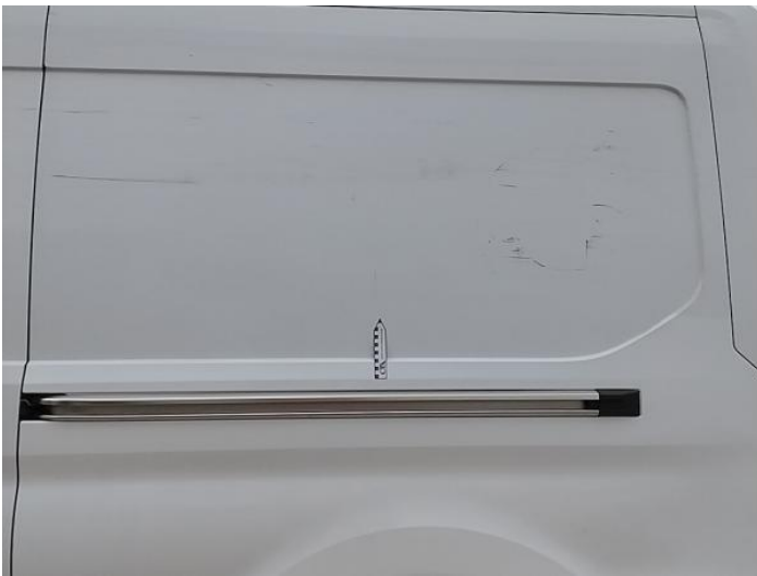
17: Qtr Panel nsr Scratched Over 25mm Not Thru Paint
