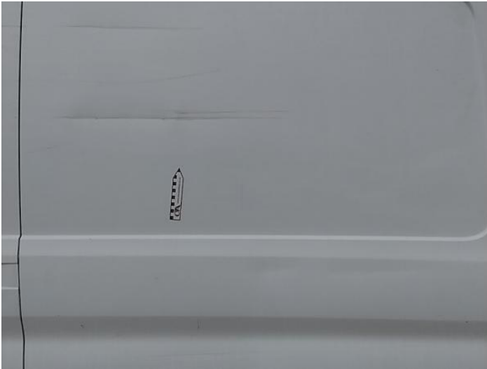
33: Qtr Panel osr Dented With Paint Damage
