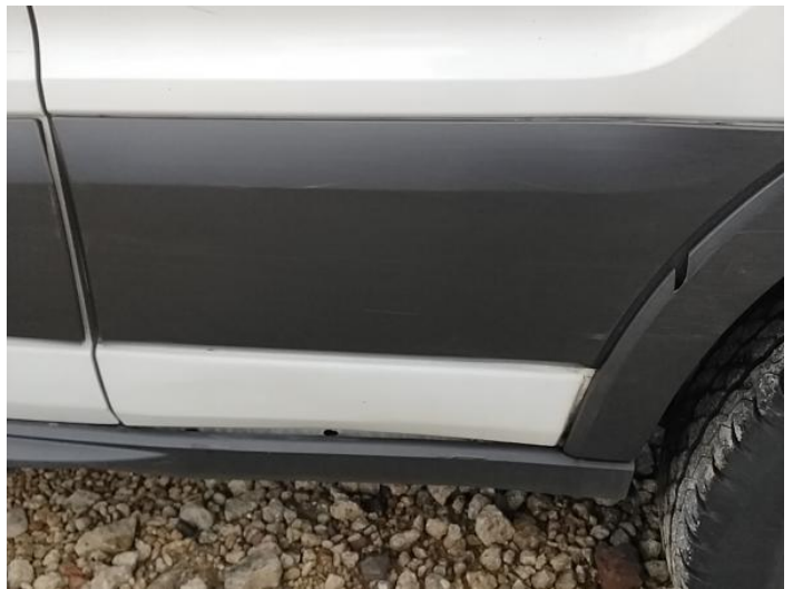
18: Qtr Panel Moulding ns Scuffed (Unpainted) UpTo 100mm
