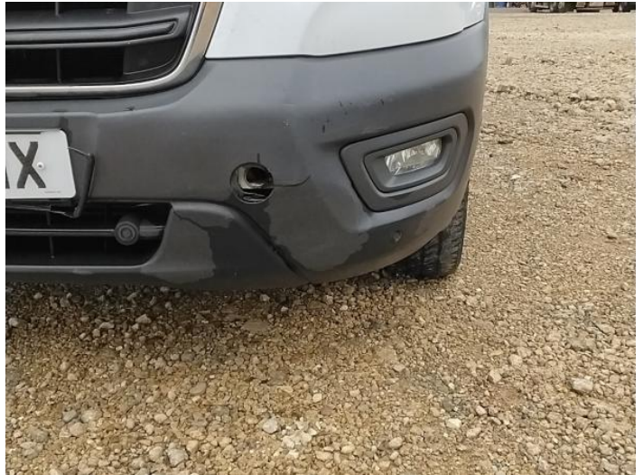
4: Front TowEye Cvr Missing Replace
