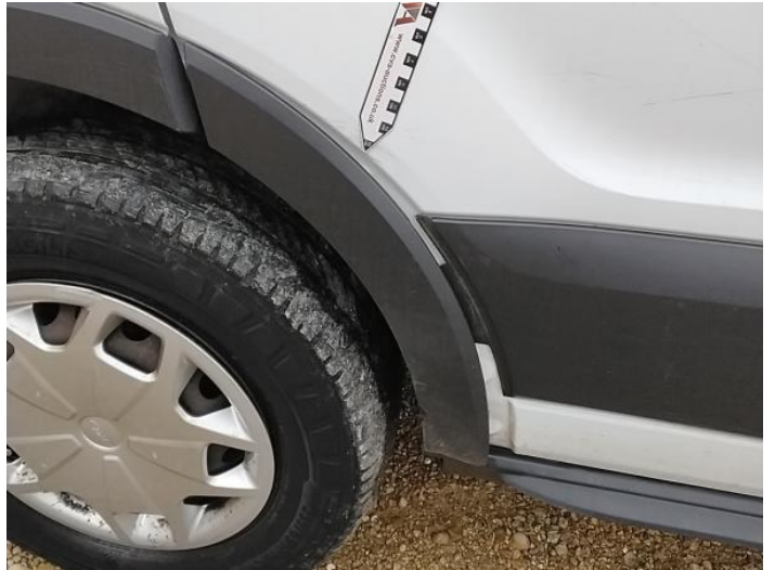
10: Moulding nsf Wing Broken Replace
