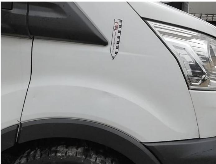
1: Wing of Dented Between 10mm + 30mm
