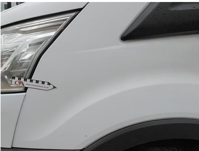
7: Wing nsf Scratched Over 25mm Not Thru Paint
