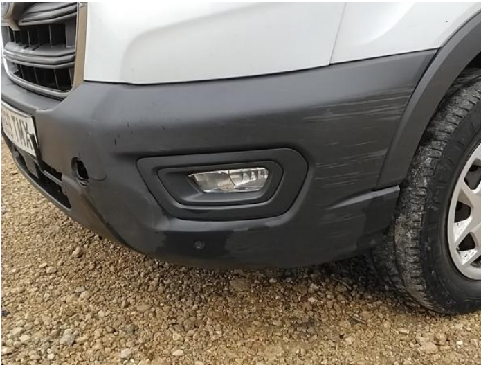
5: Bumper Front Moulding Scuffed (Unpainted) Over 100mm
