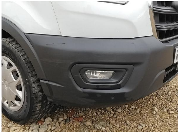
2: Bumper Front Moulding Scuffed (Unpainted) Over 100mm
