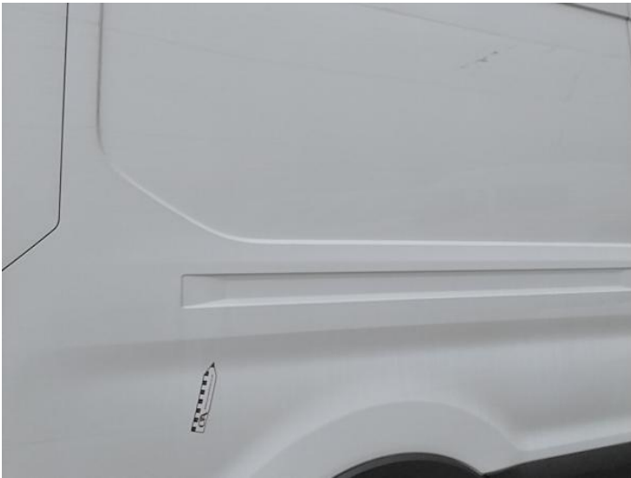
29: Qtr Panel osr Scratched Over 25mm Not Thru Paint
