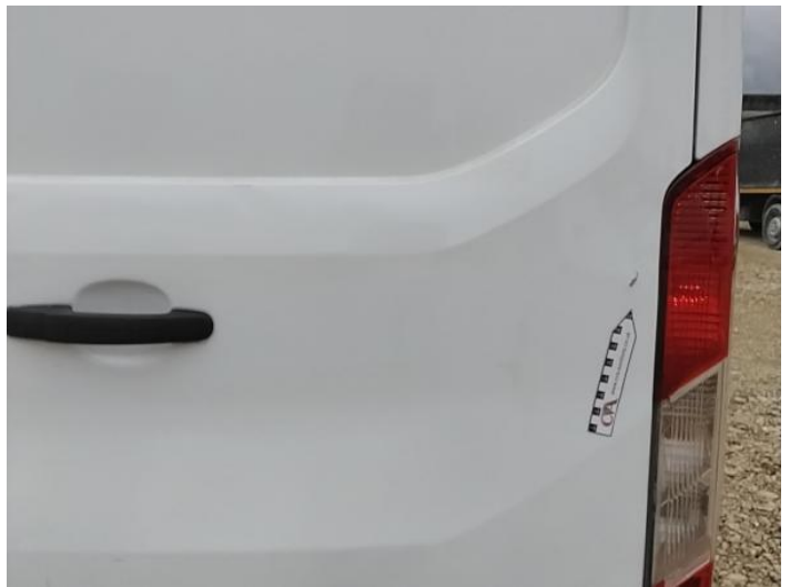
24: Door osr Dented With Paint Damage
