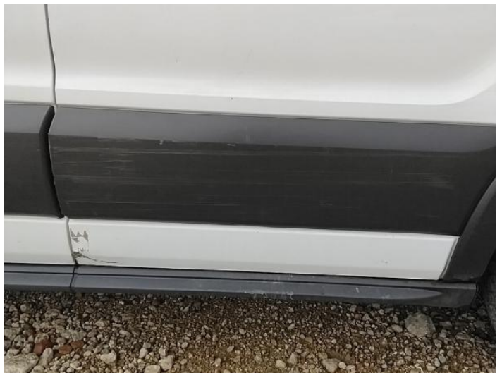
36: Door Moulding osf Scuffed (Unpainted) Over 100mm
