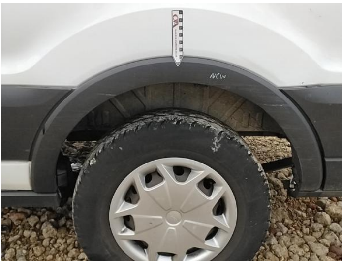
19: Qtr Panel Arch Extension ns Broken Replace
