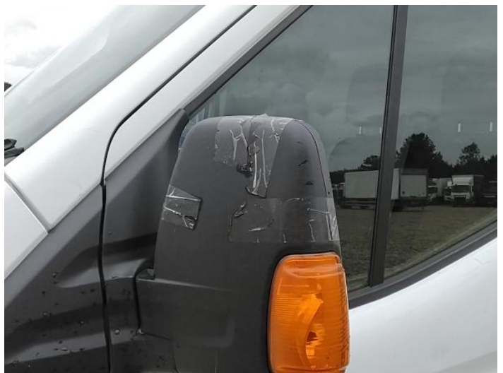
8: Door Mirror Assy nsf Broken Replace
