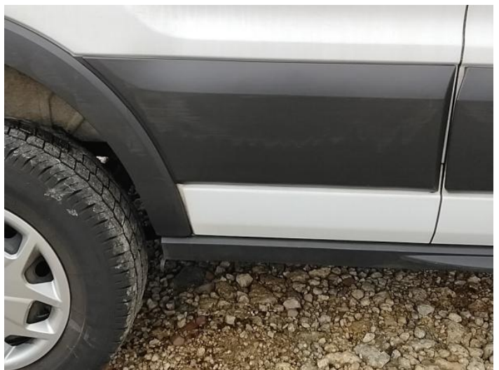
32: Qtr Panel Moulding os Scuffed (Unpainted) UpTo 100mm
