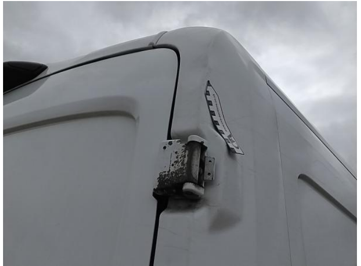
28: Panel Rear Dented Between 10mm + 30mm
