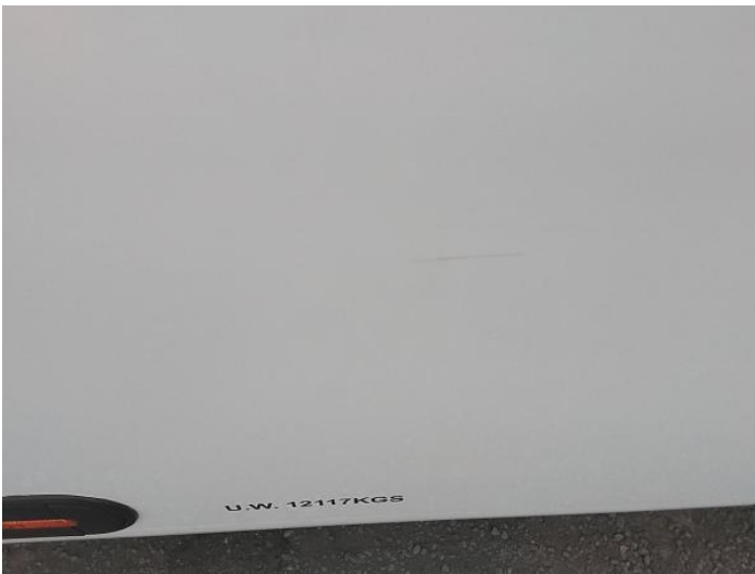
5: Qtr Panel nsr Scratched Over 25mm Not Thru Paint
