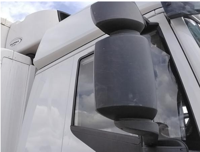
11: Door Mirror Assy osf Scuffed (Unpainted) UpTo 100mm
