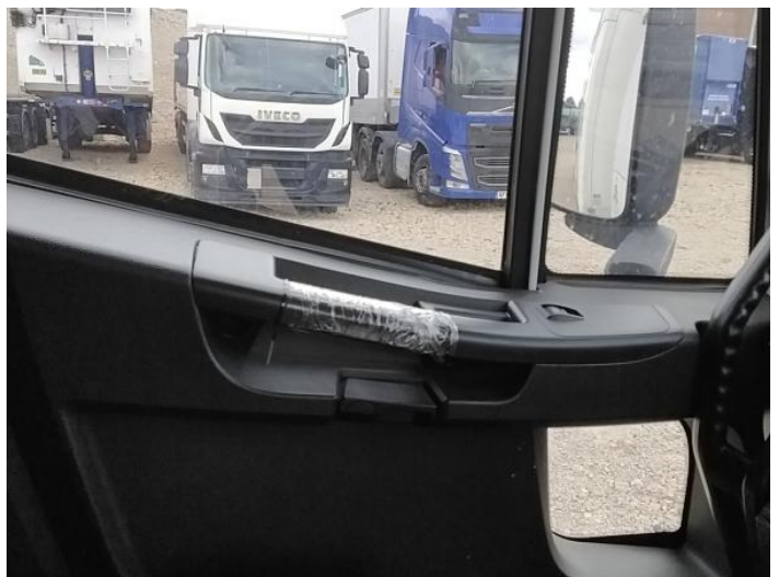
14: Handle Inner nsf Damaged Replace
