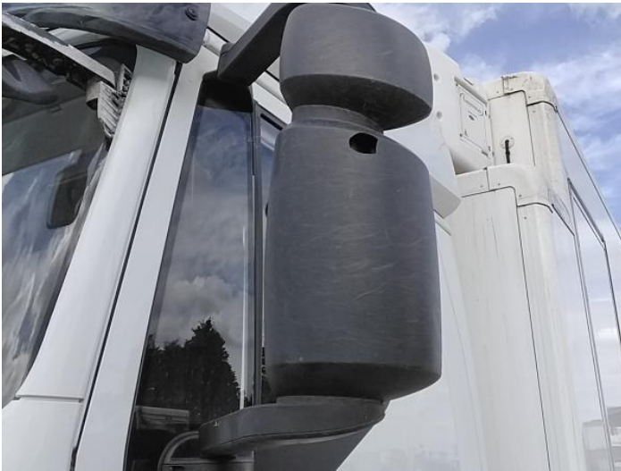
5: Door Mirror Assy nsf Broken Replace
