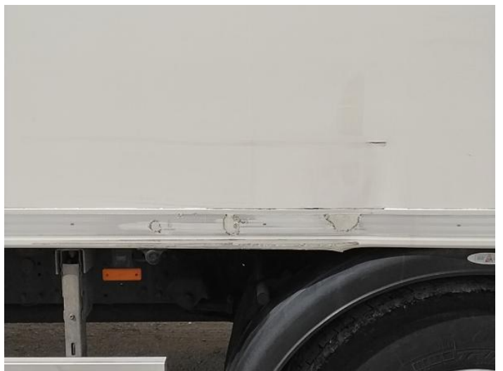
8: Qtr Panel nsr Dented With Paint Damage
