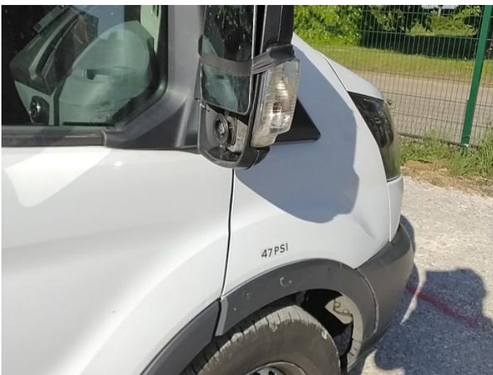
7: Door Mirror Glass os Broken Replace
