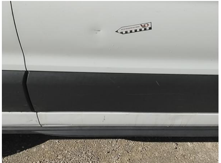
6: Door osr Dented With Paint Damage
