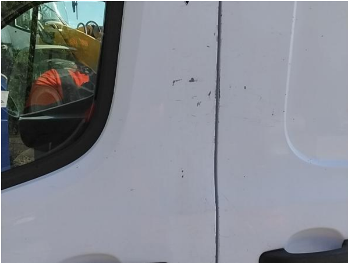
3: Door nsf Chipped Multiple Chips
