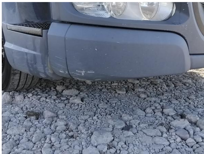
2: Bumper Front Moulding Scuffed (Unpainted) Over 100mm
