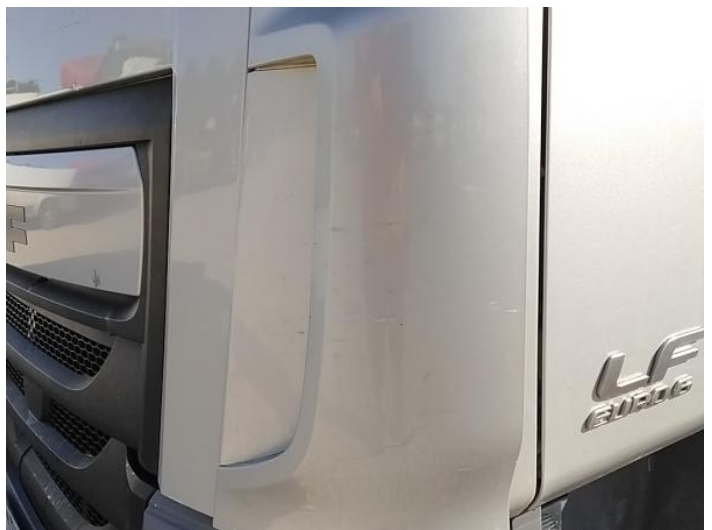
8: Wing nsf Scratched Over 25mm Thru Paint
