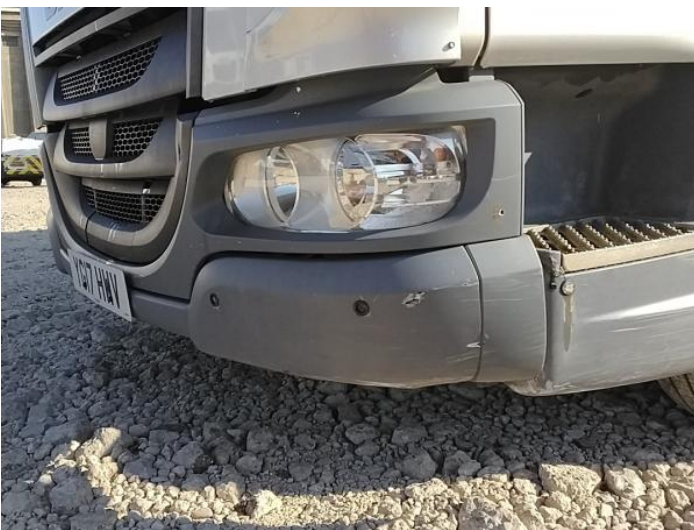
7: Bumper Front Moulding Scuffed (Unpainted) Over 100mm
