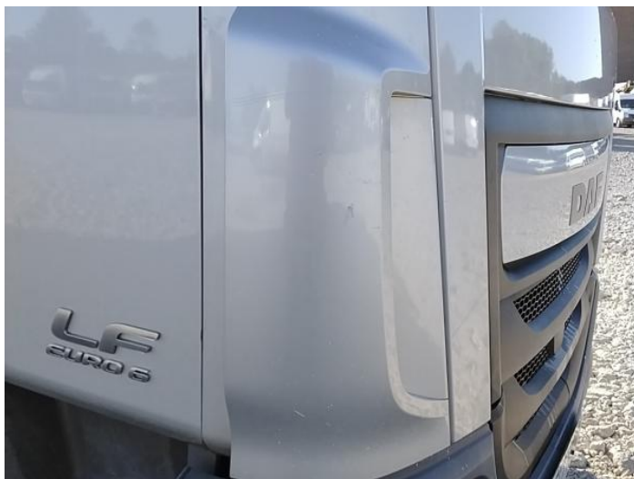
1: Wing osf Scratched Over 25mm Thru Paint
