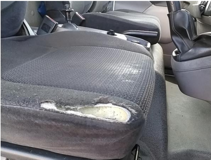
17: Seat Base Cover osf Holed Over 3mm
