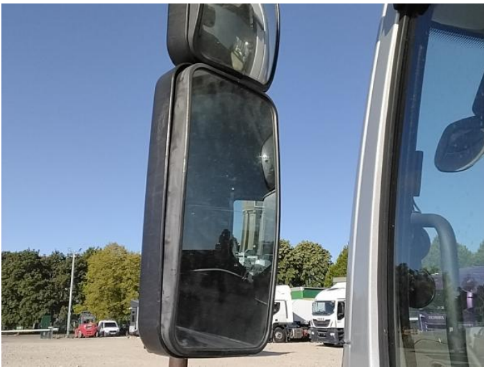
11: Door Mirror Glass ns Broken Replace
