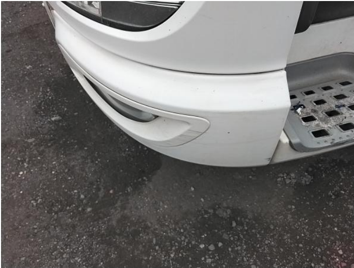
3: Bumper Front Scratched Over 100mm Thru Paint
