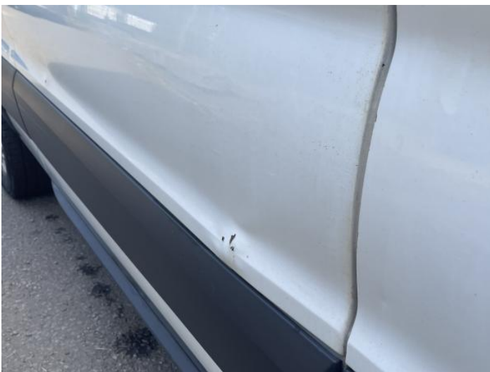
7: Qtr Panel osr Dented With Paint Damage
