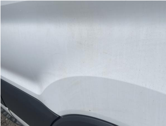
9: Qtr Panel nsr Dented Over 30mm
