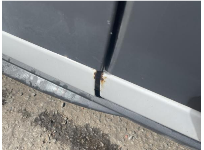
10: Door nsr Dented Over 30mm
