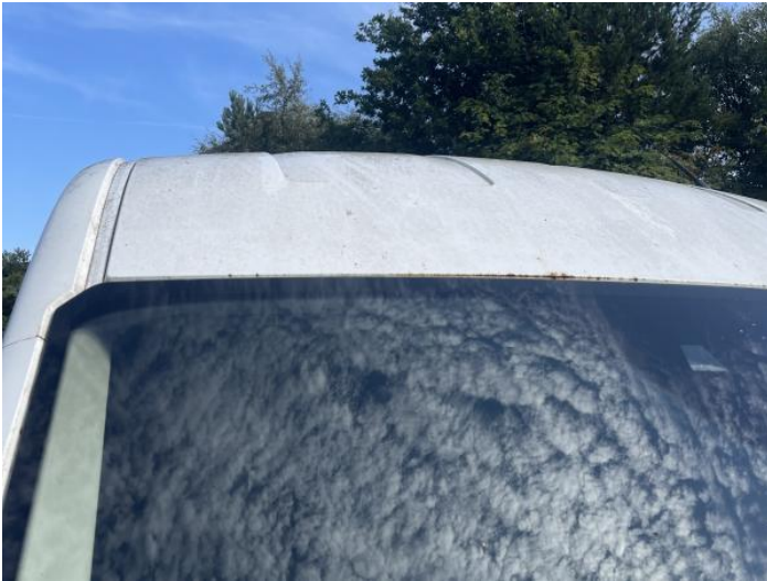
3: Roof Rusted Over 5mm
