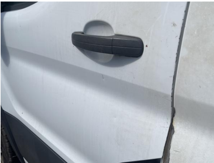
11: Door nsf Dented Over 30mm
