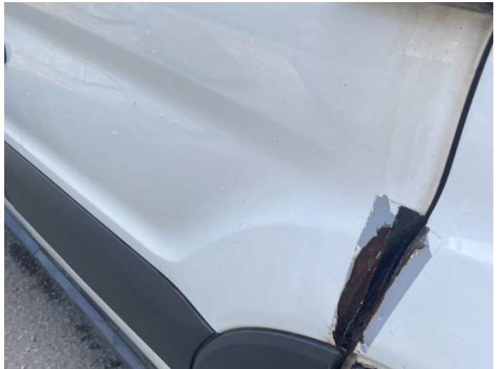
6: Door osf Dented Over 30mm
