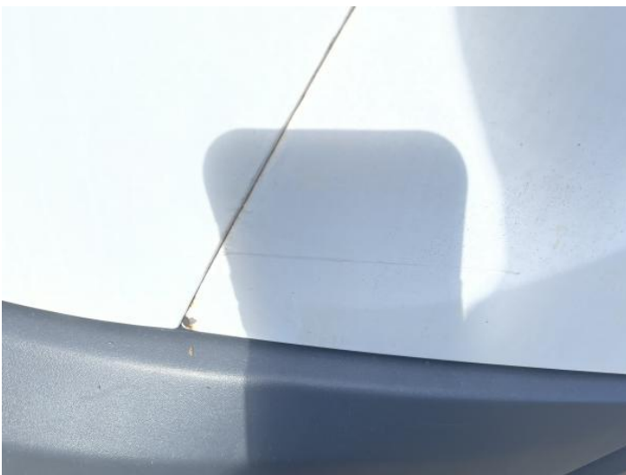
13: Wing nsf Rusted UpTo 5mm
