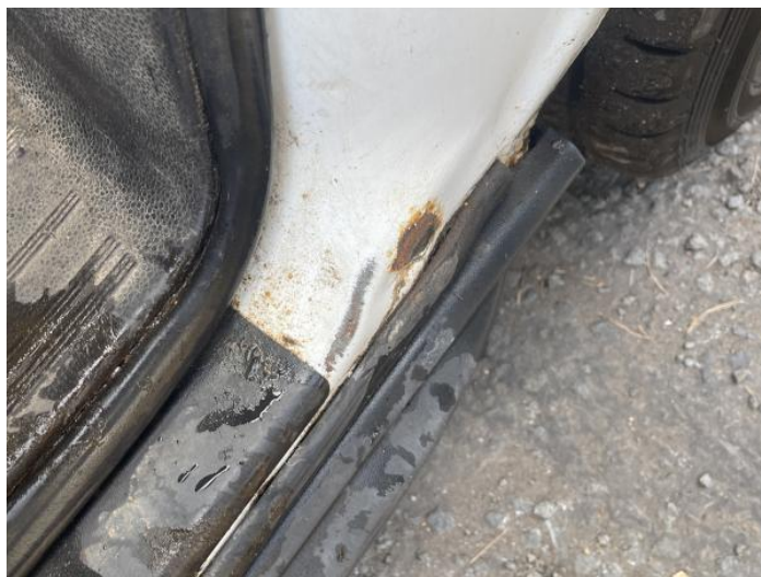
2: Sill os Rusted Over 5mm
