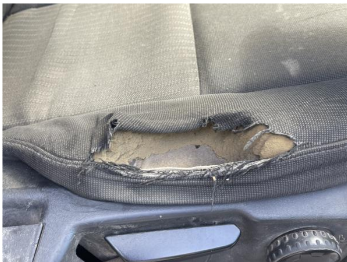
1: Seat Base Cover osf Torn Over 3mm
