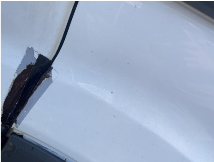
5: Wing nsf Dented With Paint Damage
