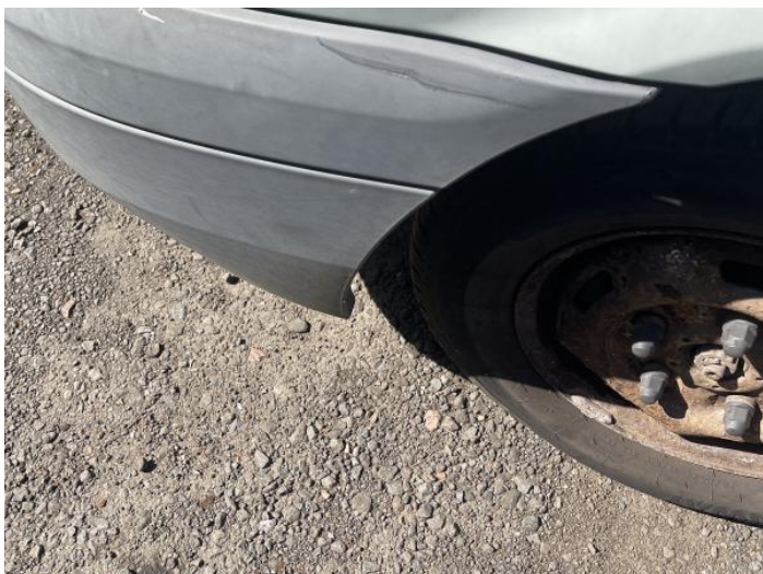
15: Bumper Front Moulding Scuffed (Unpainted) Over 100mm
