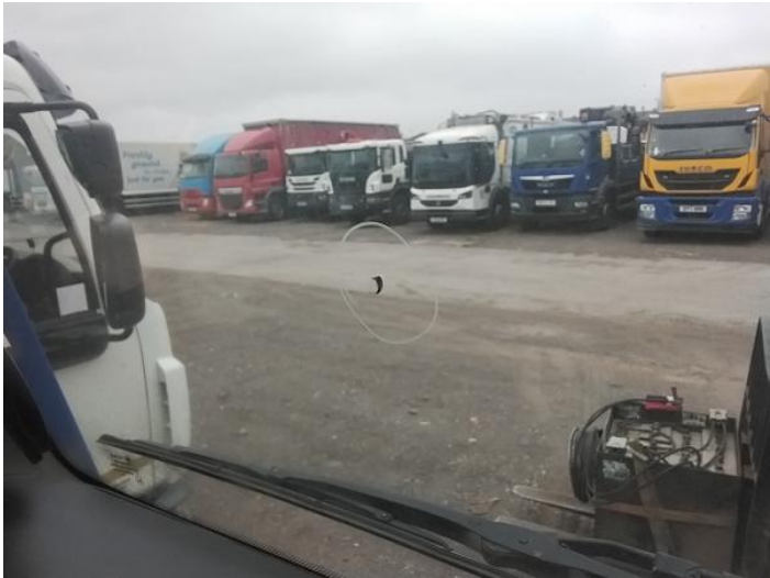
10: Screen Front Chipped Over 10mm
