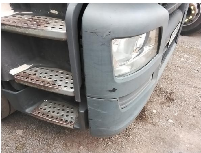
7: Bumper Front Scratched Over 100mm Thru Paint
