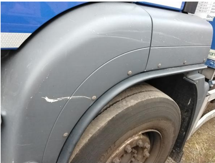
5: Wing nsf Scratched Over 25mm Thru Paint
