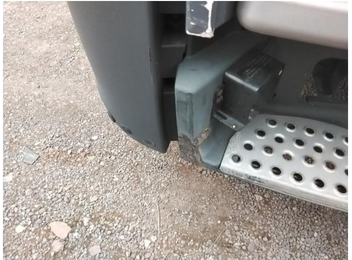
4: Bumper Front Moulding Broken Replace
