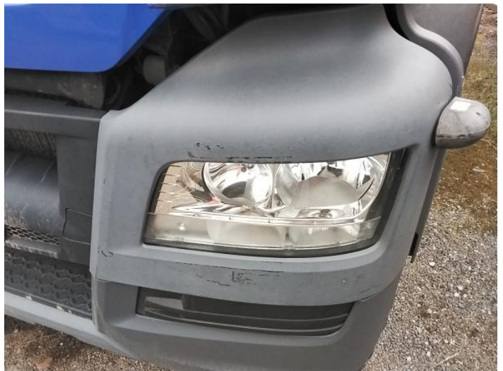
2: Panel Front Scratched Over 25mm Not Thru Paint
