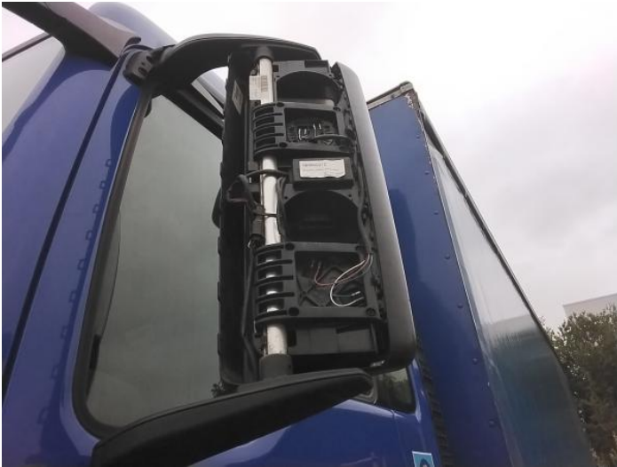
3: Door Mirror Assy nsf Broken Replace
