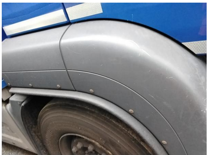
8: Wing osf Scratched Over 25mm Thru Paint
