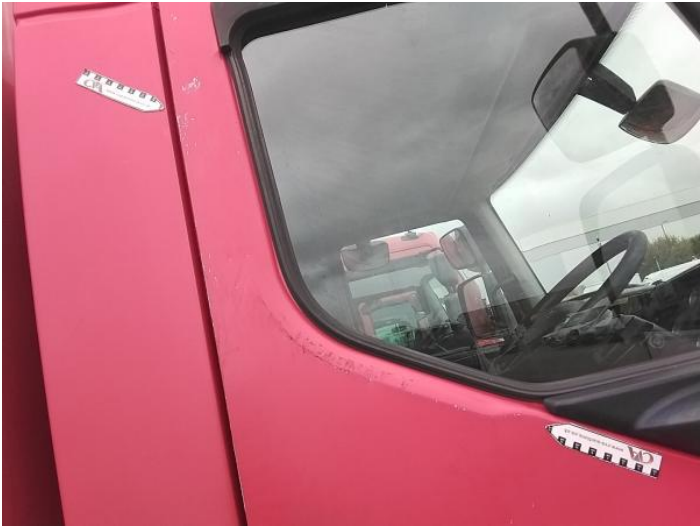
3: Door osf Scratched Over 25mm Thru Paint
