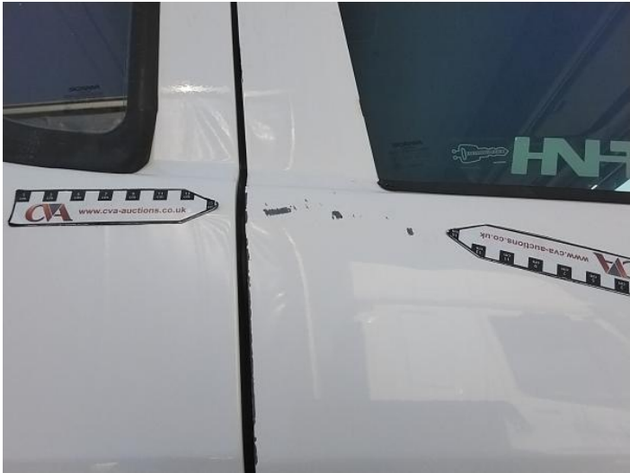
4: Door osf Dented With Paint Damage
