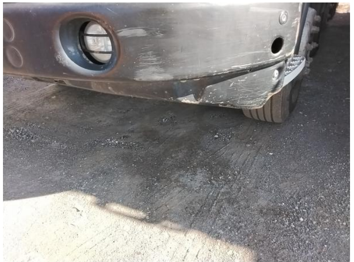
2: Bumper Front Dented With Paint Damage
