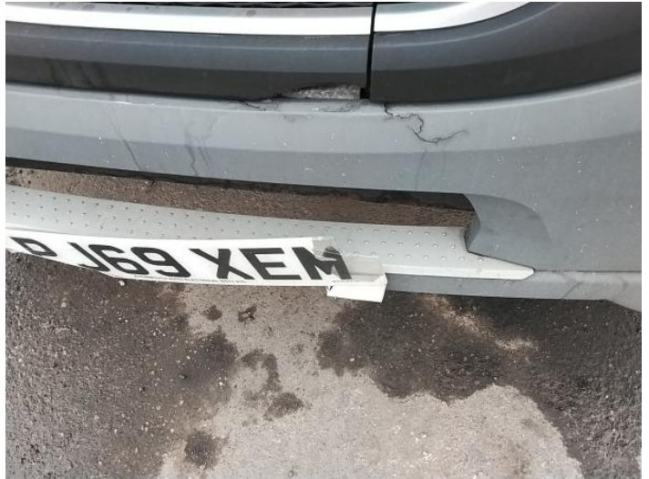
4: Bumper Front Cracked Over 25mm
