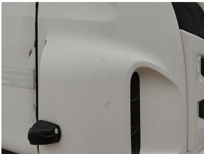
1: Wing osf Scratched UpTo 25mm Thru Paint
