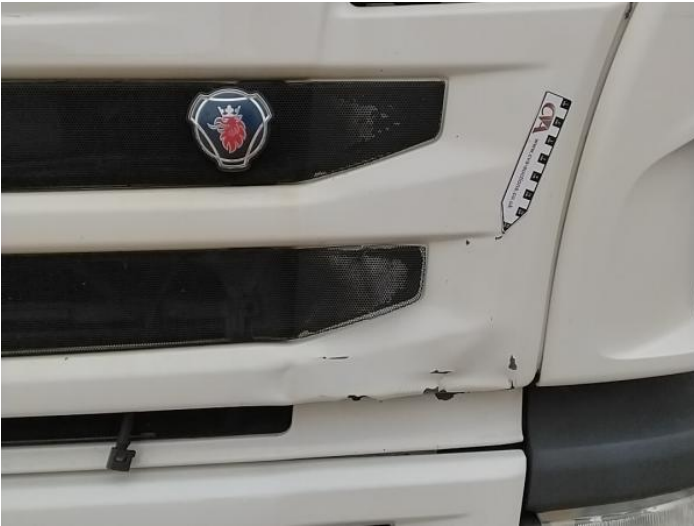
3: Bonnet Dented With Paint Damage
