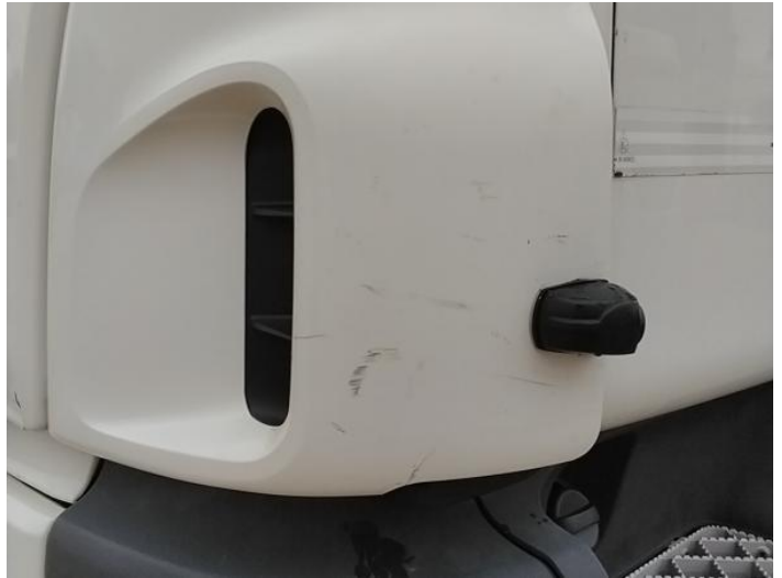
4: Wing nsf Scratched UpTo 25mm Thru Paint
