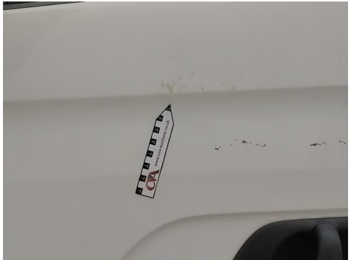
6: Door nsf Scratched UpTo 25mm Thru Paint
