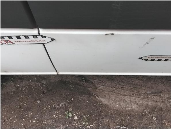
15: Qtr Panel osr Dented With Paint Damage
