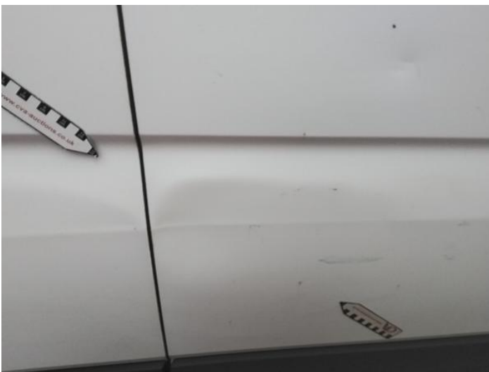
13: Qtr Panel osr Dented Over 30mm
