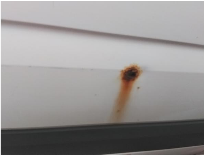
17: Qtr Panel osr Rusted Over 5mm
