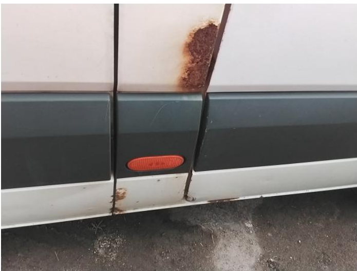
19: B Post os Rusted Over 5mm
