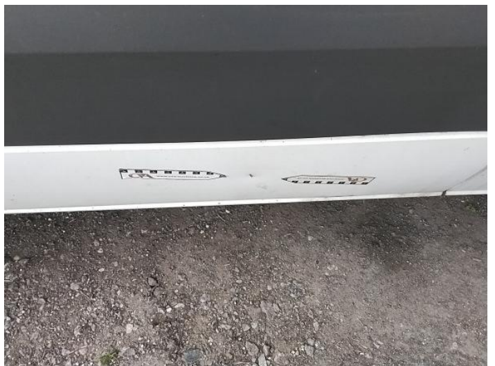
8: Qtr Panel nsr Dented With Paint Damage
