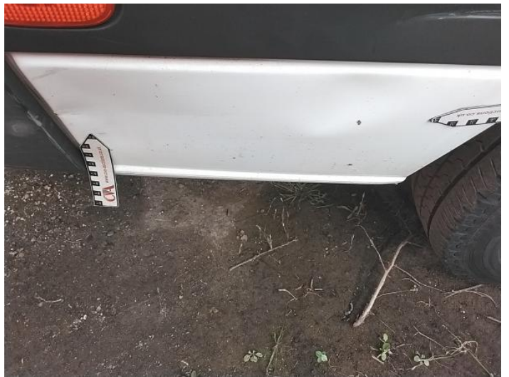
12: Qtr Panel osr Dented With Paint Damage
