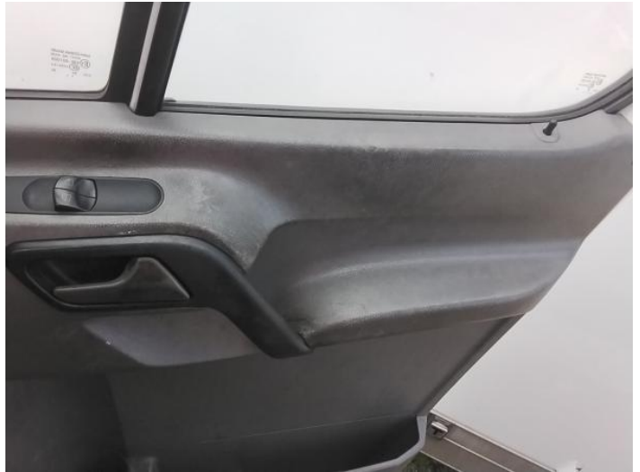
22: Door Pad osf Soiled Heavy
