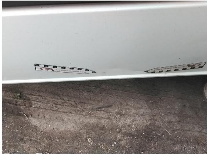
16: Qtr Panel osr Dented Over 30mm
