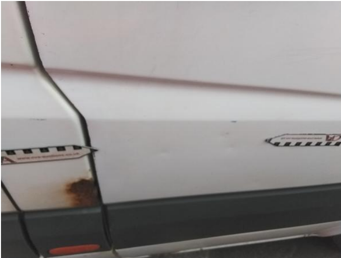
21: Door osf Dented With Paint Damage
