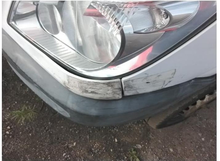
4: Wing nsf Poor Previous Repair Poor Paint
