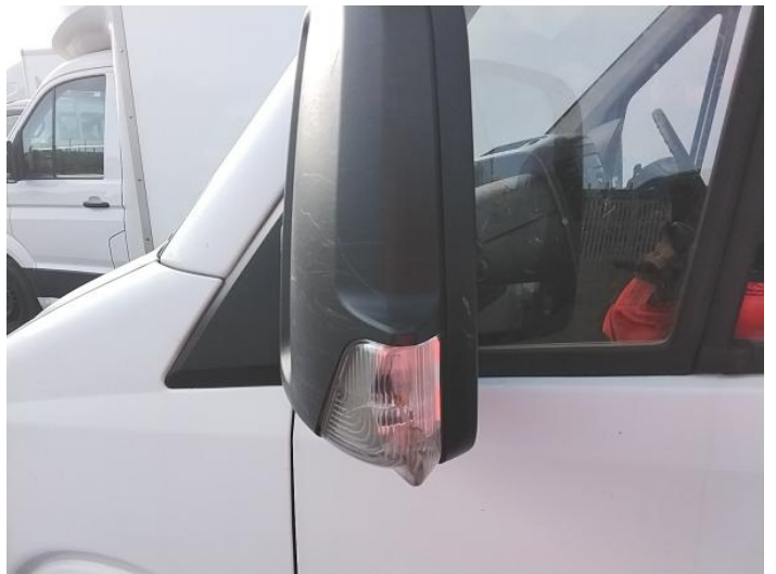
6: Door Mirror Assy nsf Broken Replace
