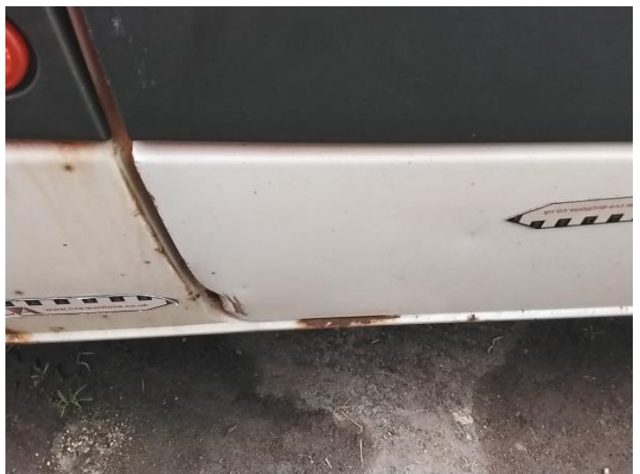
20: Door osf Dented With Paint Damage
