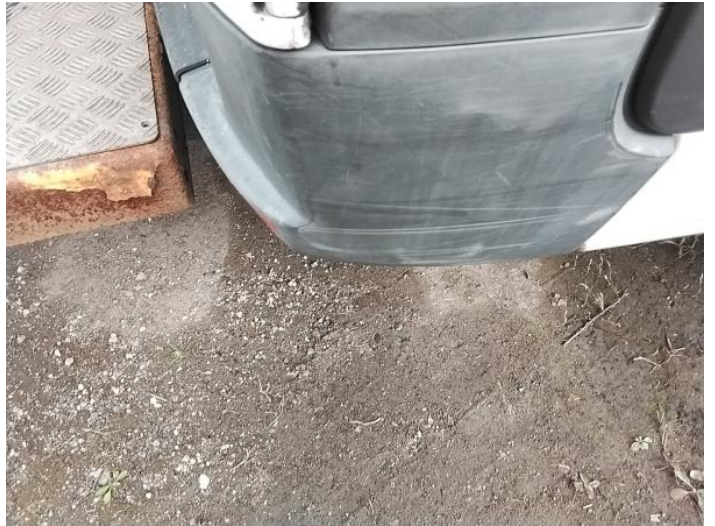
10: Bumper Rear Moulding Scuffed (Unpainted) Over 100mm
