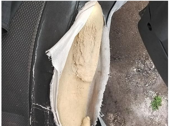
24: Seat Base Cover osf Torn Over 3mm
