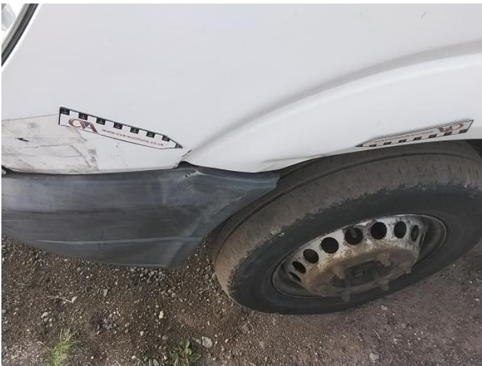
5: Wing nsf Dented With Paint Damage
