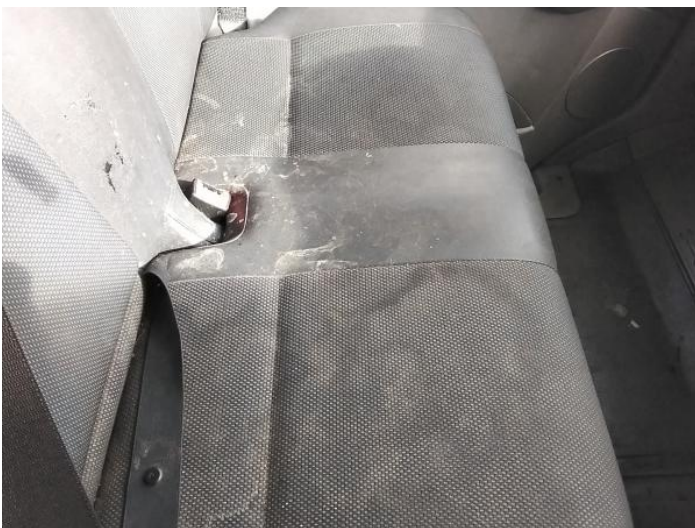
25: Seat Base Cover nsf Soiled Heavy
