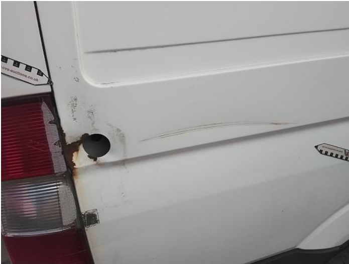
9: Qtr Panel osr Dented With Paint Damage
