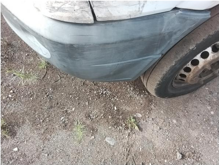
3: Bumper Front Scratched Over 100mm Thru Paint
