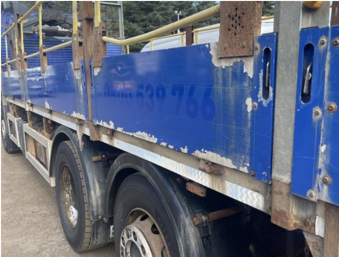
9: Qtr Panel nsr Dented With Paint Damage
