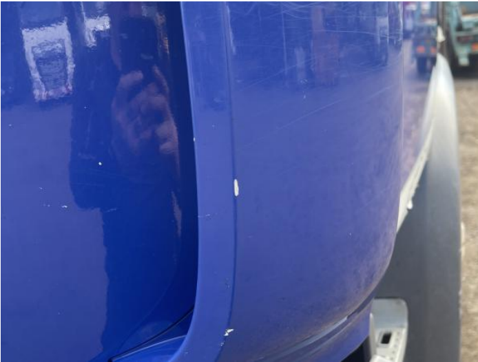
3: Wing nsf Chipped Multiple Chips
