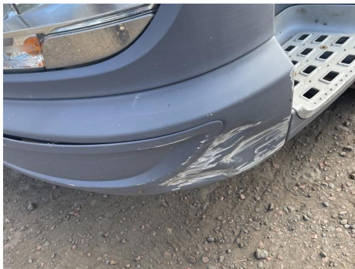
2: Bumper Front Moulding Scuffed (Unpainted) Over 100mm
