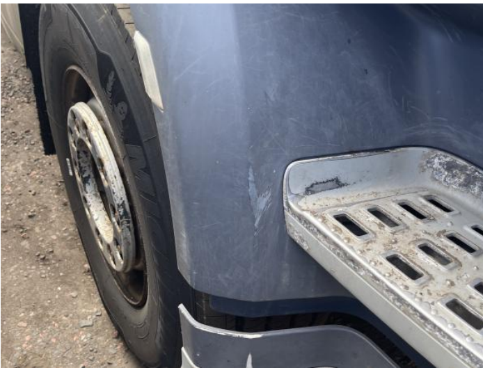
5: Door Moulding osf Scuffed (Unpainted) Over 100mm
