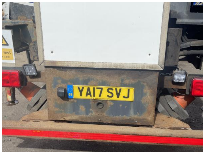
8: Tailgate Rusted Over 5mm
