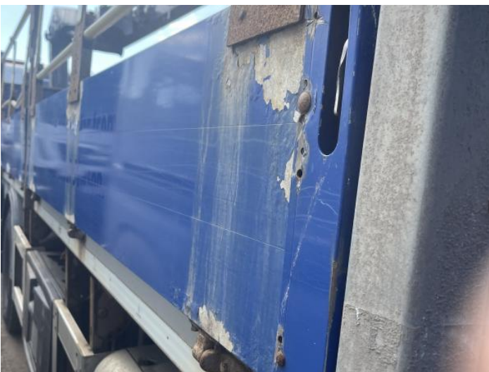
7: Qtr Panel osr Rusted Over 5mm
