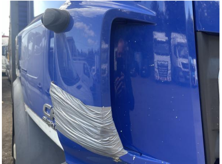
4: Wing osf Cracked Replace
