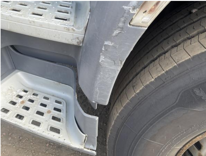
11: Door Moulding nsf Scuffed (Unpainted) Over 100mm
